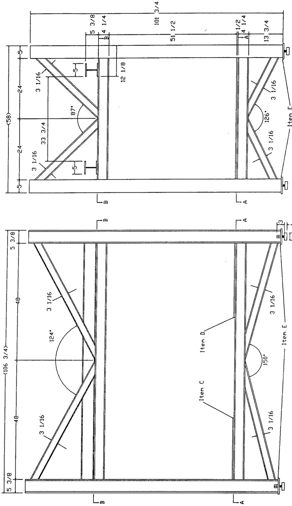
Materials Of Construction: 5 Inch H Beams, 4 Inch H Beams, 3 Inch I Beams, 1/2 Inch Thick Plate.
