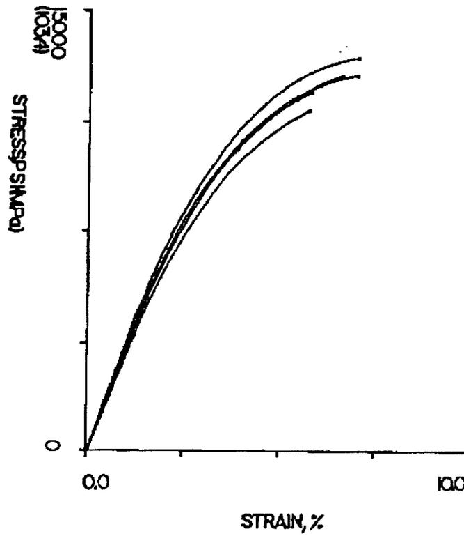
Run 72 EXPOSED Stress Versus Strain Curves:
