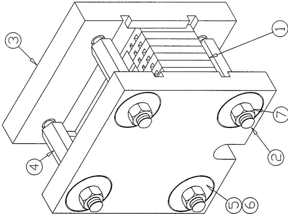
Figure 13: Mold Pack: Assembly
