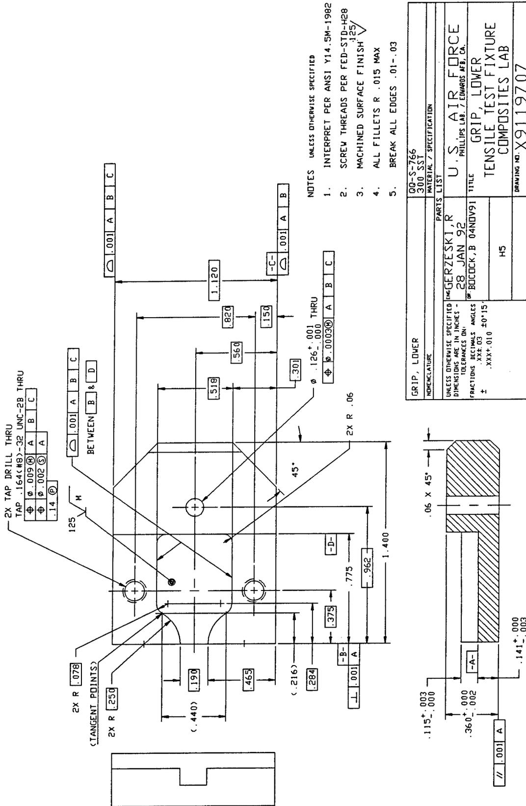
Figure A40: Tensile Test Fixture: Lower Grip
