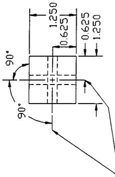
Ream Two Intersecting Crossed 0.250" Dia Dowel Pin Holes As Shown At All Four B--B Sections
