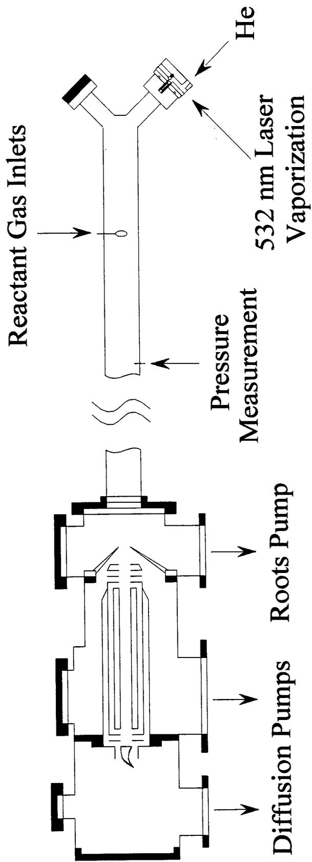
Figure 2-5: Schematic drawing of fast flow tube.
