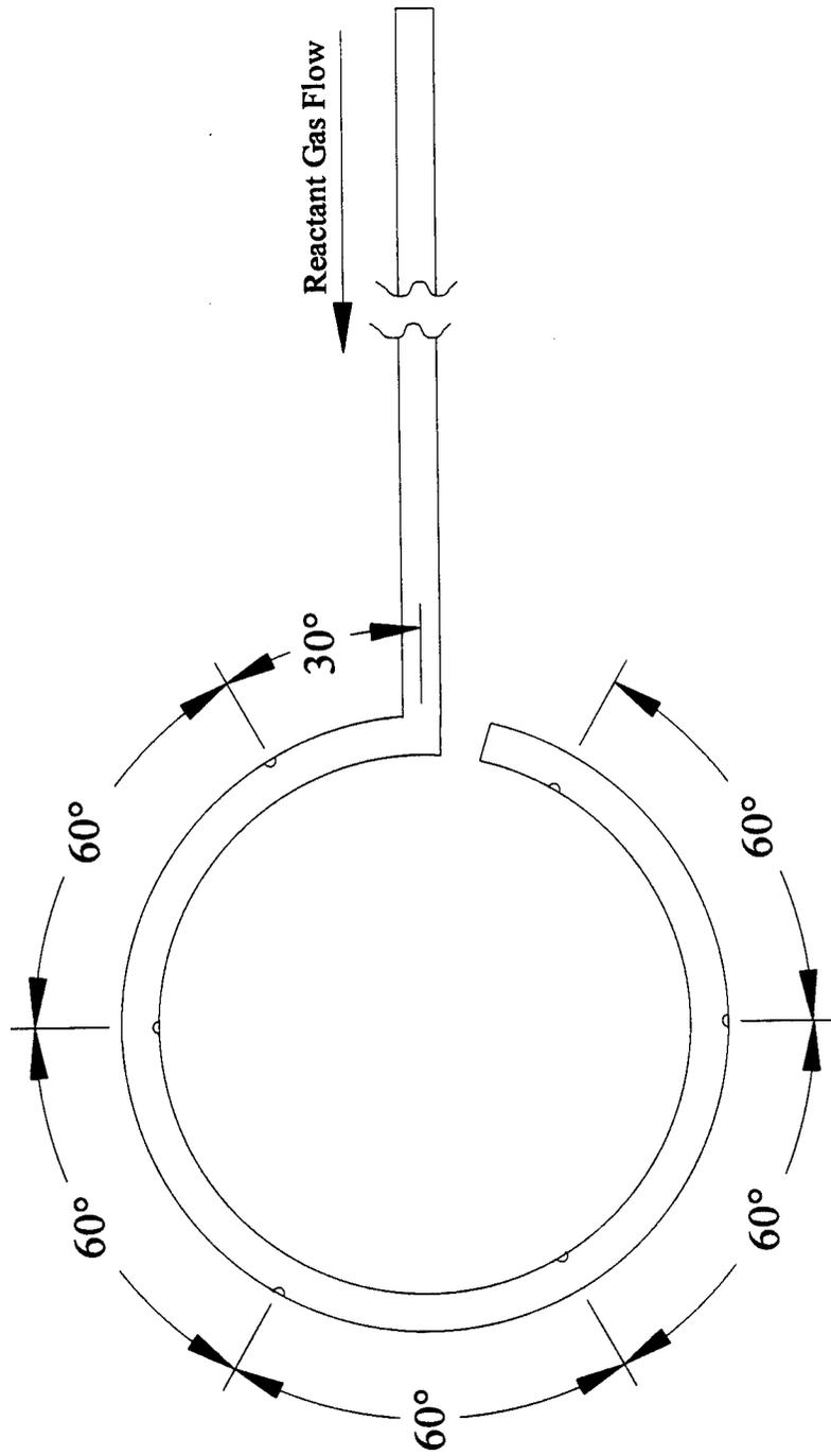
**Figure 2-6:** Schematic drawing of the reactant gas inlet (RGI). Each 0.4 mm hole is located 60° apart. Three holes point radially inward and three holes point radially outward.
