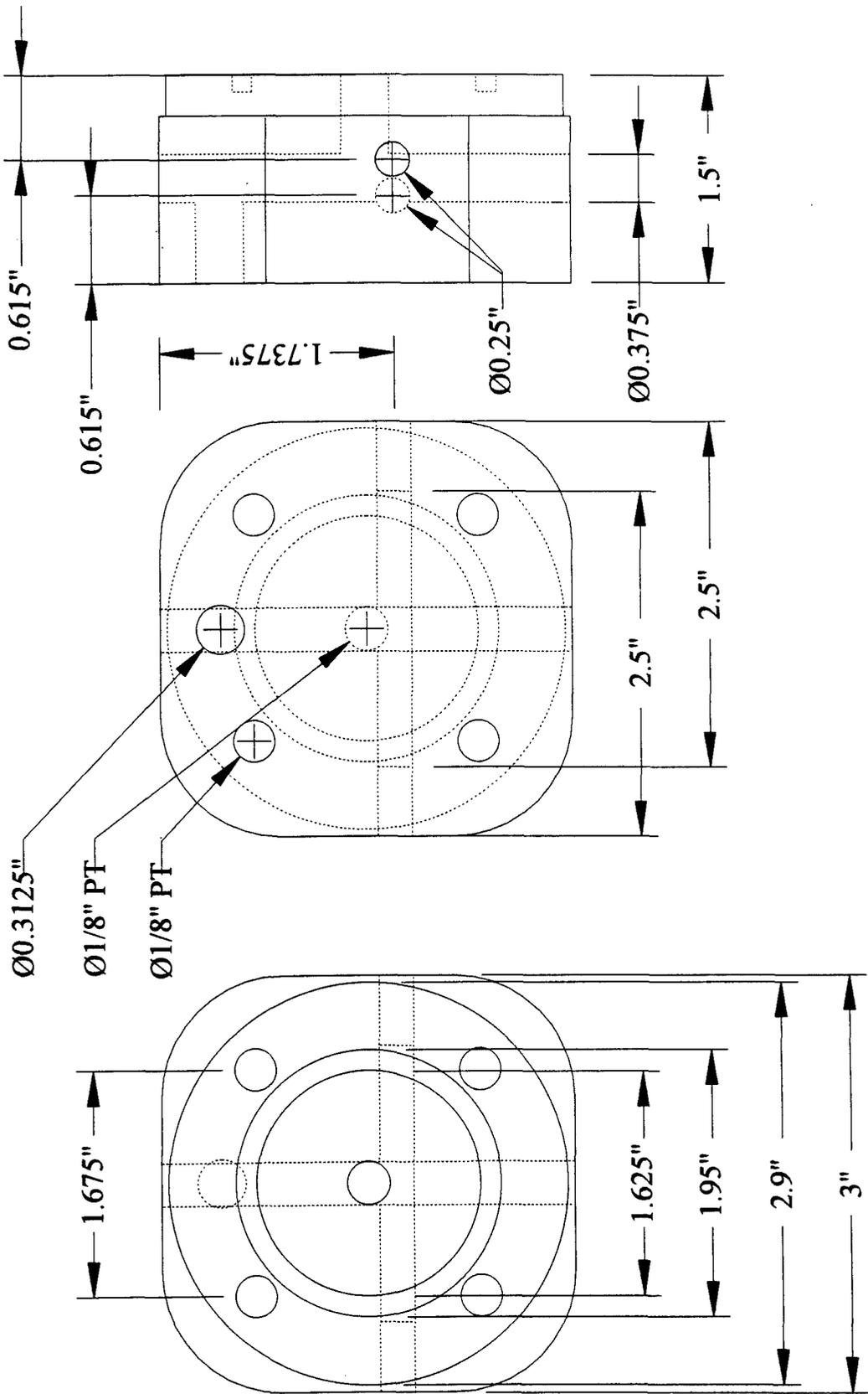
Figure 2-3: Dual rod LAVA source specification diagram.
