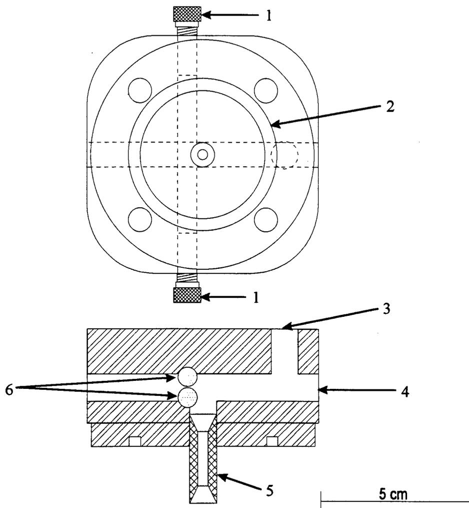
*Figure 2-4:* Horizontal cross section and front view of the new dual rod LAVA source. (1) Ultra-Torr fittings housing the target rods and allowing for rotation while maintaining vacuum. (2) O-ring groove. (3) Carrier gas inlet. (4) Laser beam channel. (5) Teflon nozzle with a 1/8 in. dia. bore. (6) Target rods, 0.0200 in. apart.
