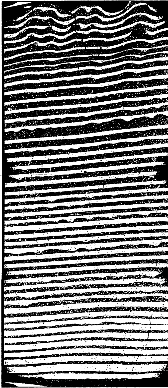
Fig. 24: Cross-section of \text{Al}_2\text{O}_3/\text{ZrO}_2 laminar composite
