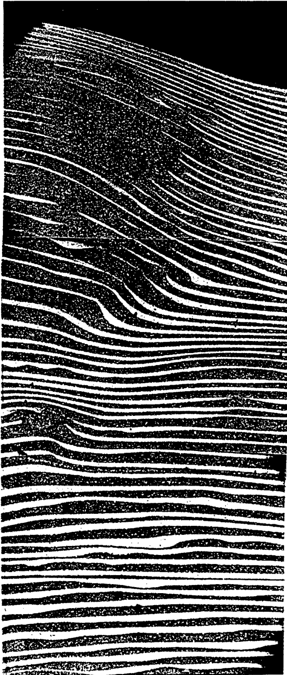
Fig. 30 : Cross-section of a \text{ZrO}_2/\text{Al}_2\text{O}_3 + \text{ZrO}_2 laminar composite deposited from a \text{ZrO}_2 suspension and from a 96% w \text{Al}_2\text{O}_3 + 4\% w \text{ZrO}_2 suspension
