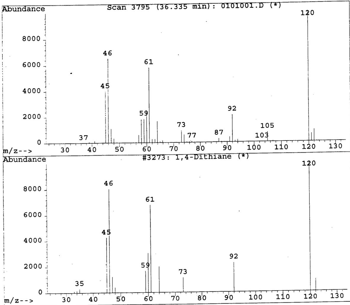
**Figure 4.25.** Mass Spectral Signature of 1,4-Dithiane as Desorbed (upper panel) and in NBS Library (lower panel)
