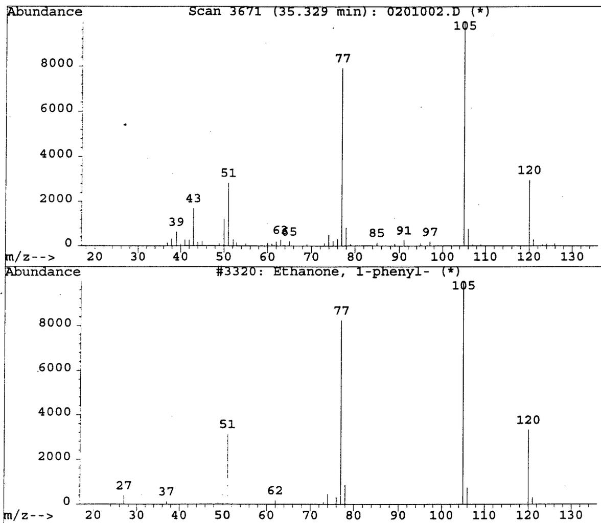
**FIGURE 4.21.** Acetophenone in G Street GS1 Hive Sample of August 23, 1996 (top panel), compared to NBS Library Spectrum (bottom panel)
