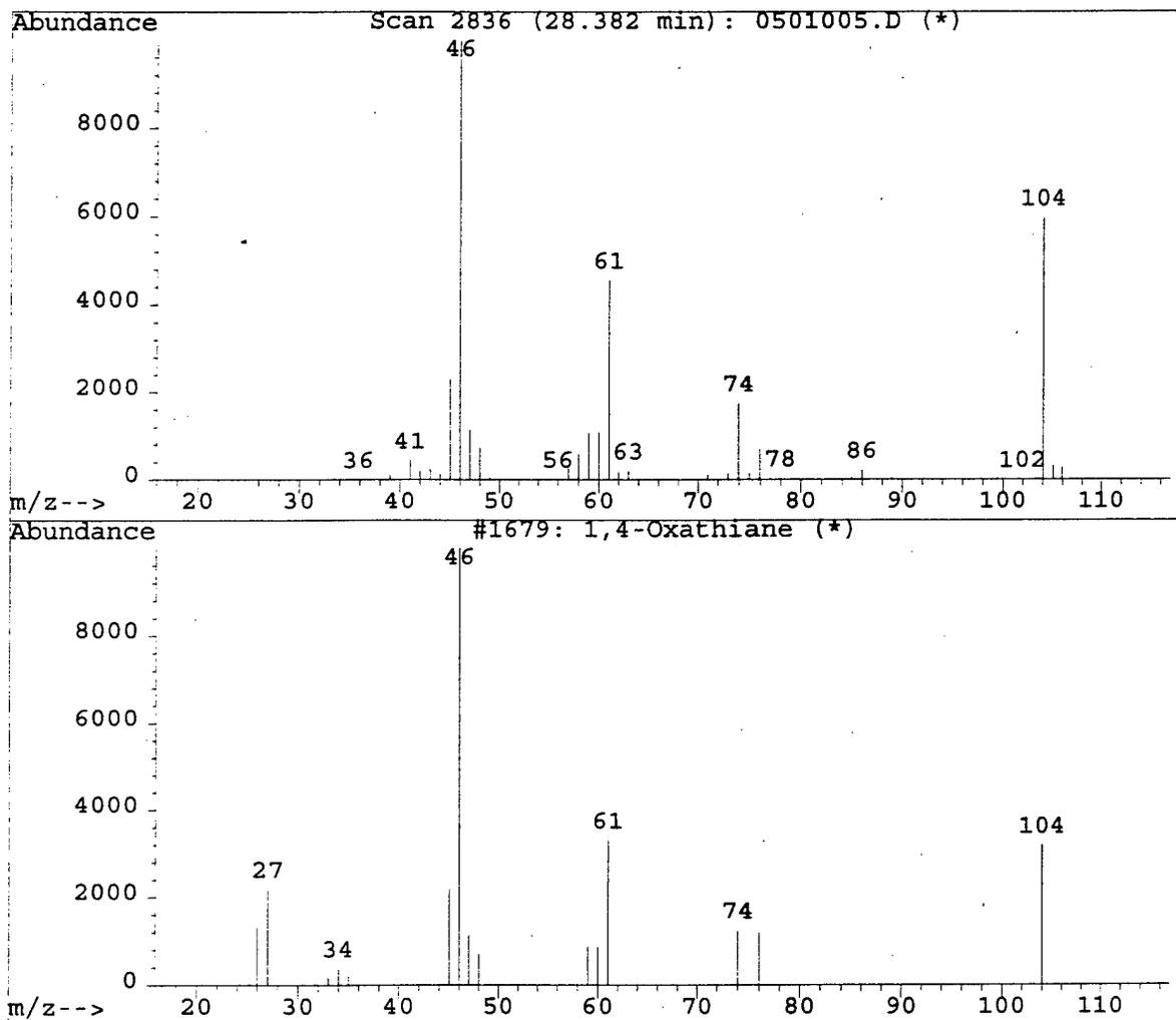
**Figure 4.24.** Mass Spectral Signature of 1,4-Oxathiane in Thiodiglycol (upper panel) and NBS Library (lower panel)
