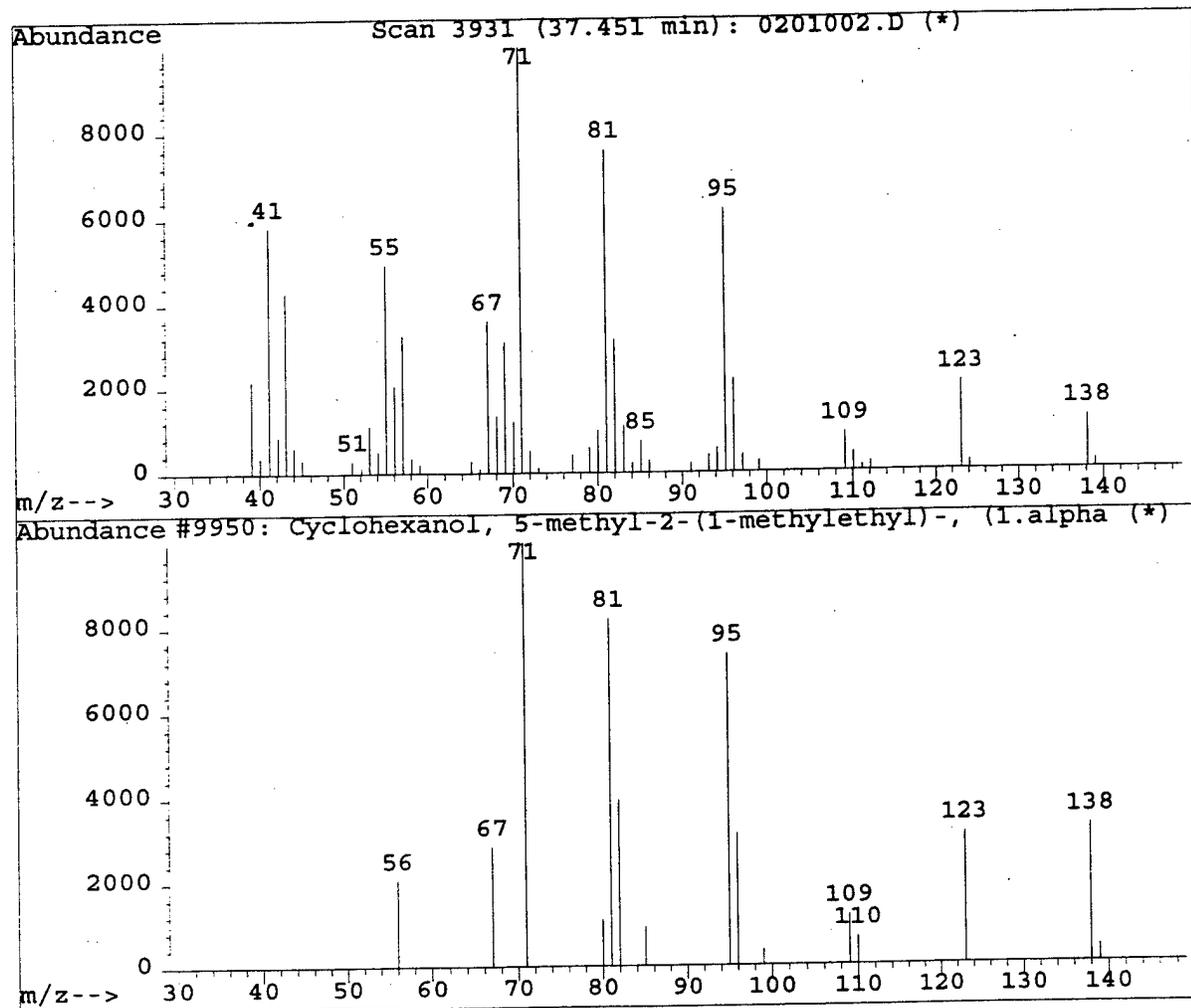
Figure 4.28. Menthol in August 18 Sample from West Branch Canal Creek Condo 2 (upper panel) and NBS Library Spectrum (lower panel)
