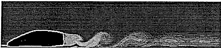
Figure 15: Flow over the Mercedes Benz 2-D Automobile Model Computed Using the RNG K-\epsilon Model.
