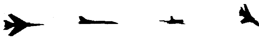
Figure 8; Various aspects of a Tu-26 (Backfire) bomber generated with the model generator.
