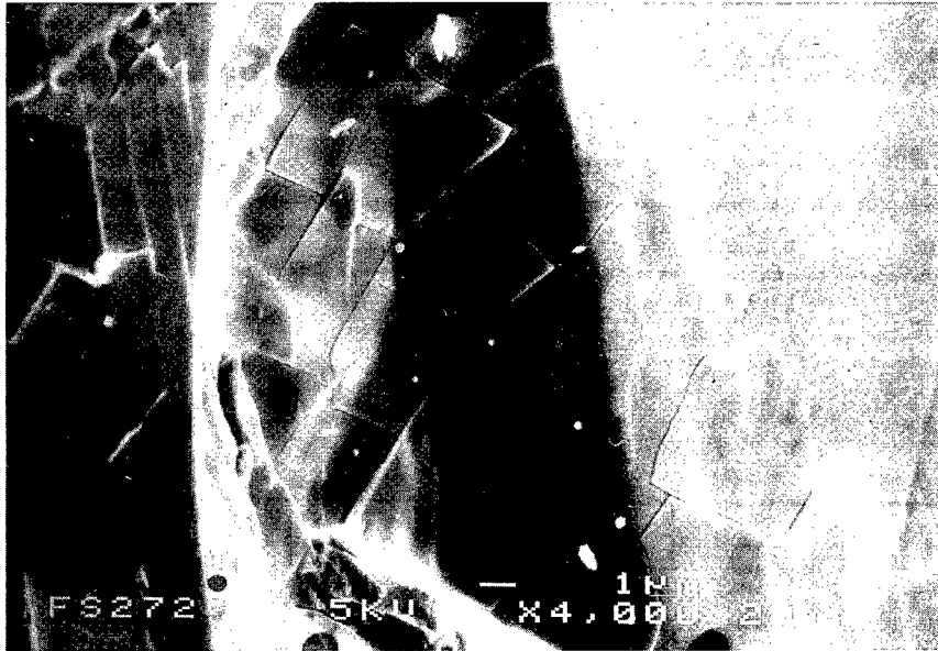
FIGURE 1(c) SE micrograph illustrating 'massive' damage at 11.7 J/cm 2 .
