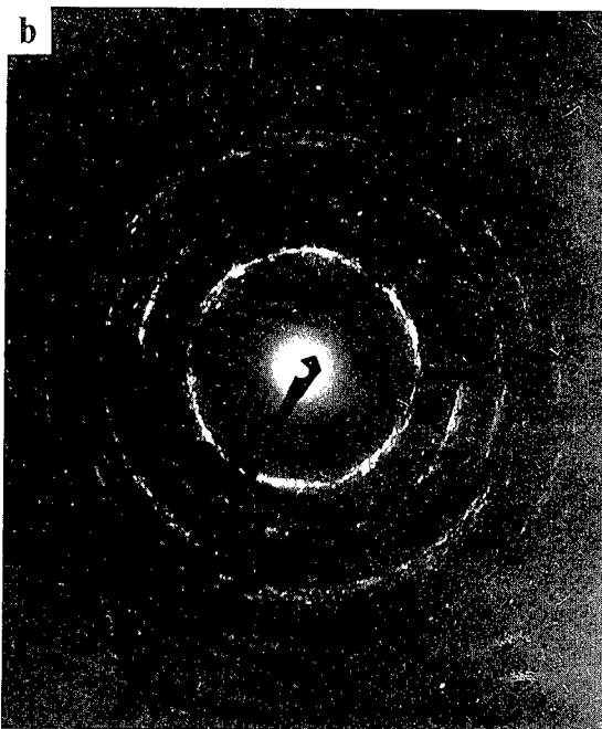
Figure 3: Microstructure of the Zr -20 at.% Zn alloy obtained by mechanical alloying under pressure: (a) TEM bright-field image; (b) selected area diffraction pattern corresponding to (a).
