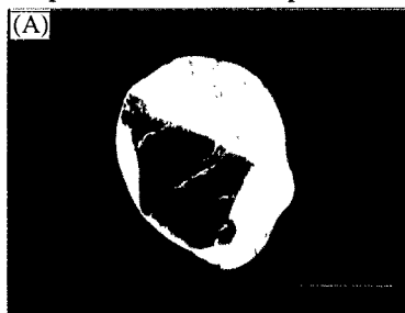
Fig. 1 (A) Photomicrograph of graphite sample at 14.4 GPa in a DAC with a transmitted light before laser heating. Scale bar is 0.1mm.
