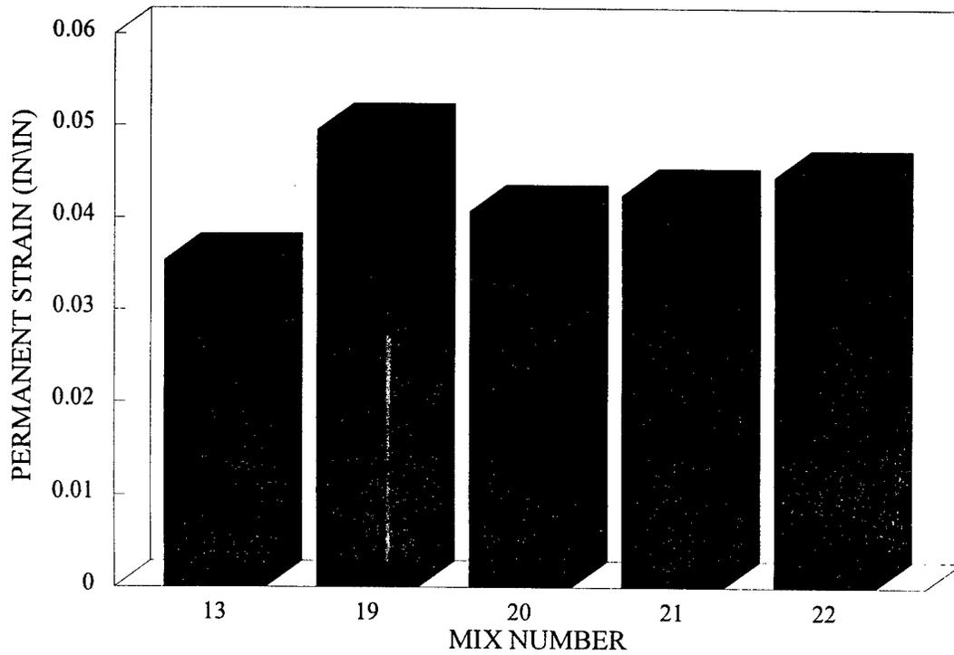
FIGURE 26. EFFECTIVE OF CRUSHED COARSE AGGREGATE ON PERMANENT STRAIN VALUES FOR AC-20 MIXTURES
