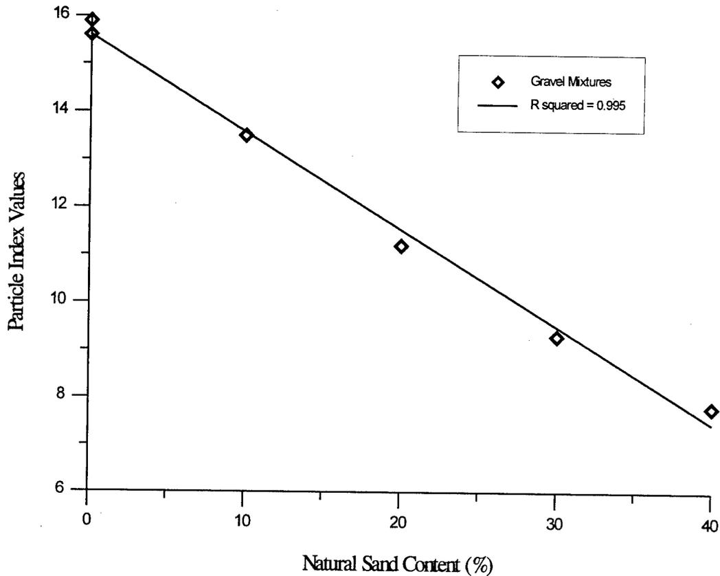
FIGURE 14. PARTICLE INDEX VALUES VERSUS NATURAL SAND CONTENT
