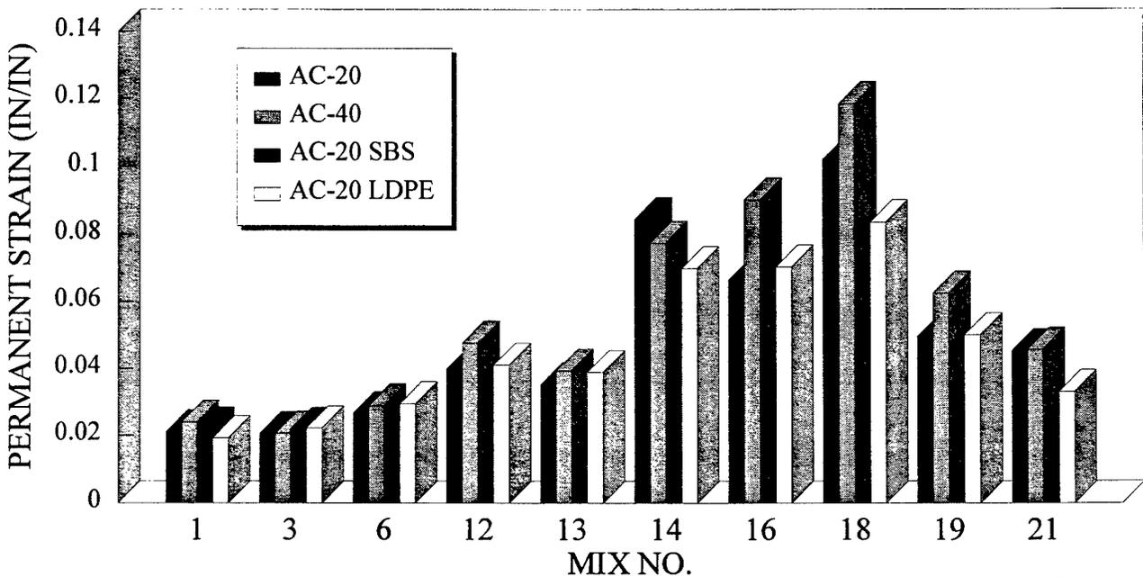
FIGURE 41. EFFECT OF STIFF ASPHALT BINDERS ON PERMANENT STRAIN VALUES
