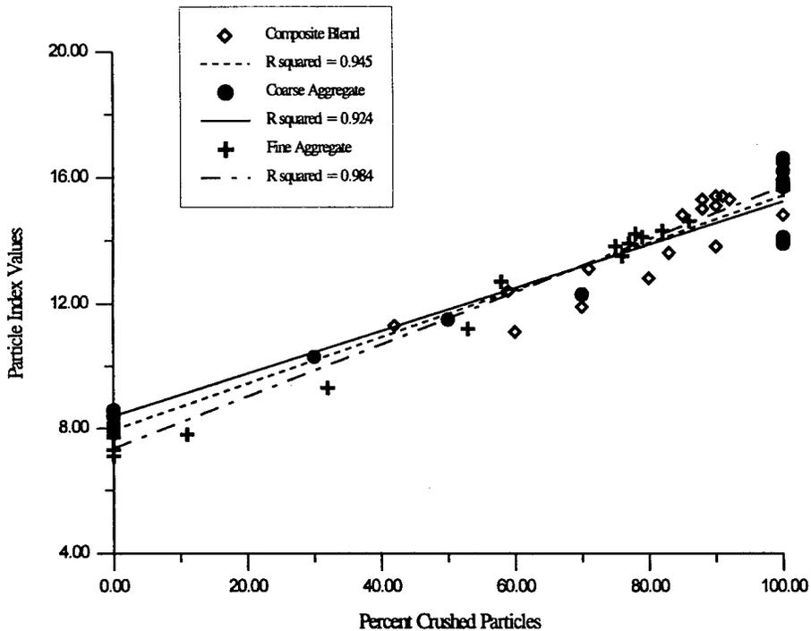
FIGURE 9. PARTICLE INDEX VALUES VERSUS PERCENT CRUSHED PARTICLES
