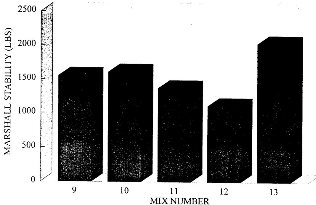
FIGURE 28. EFFECT OF NATURAL SAND CONTENT ON MARSHALL STABILITY VALUES FOR AC-20 MIXTURES
