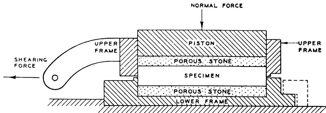
FIGURE 3. SCHEMATIC DIAGRAM OF DIRECT SHEAR BOX [16]
