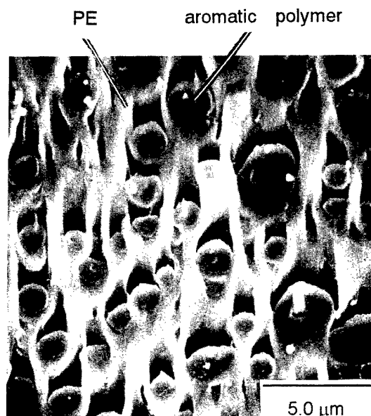
Figure 2 Morphology of the blend of aromatic polymer and PE
