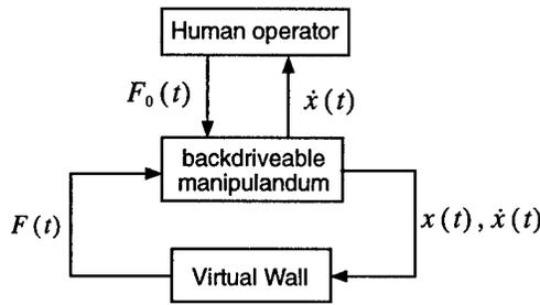
**FIGURE 7. Block diagram description of virtual contacting environment.**
