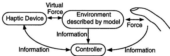
**FIGURE 2. The communication paths of electro-magnetic haptic interface.**
