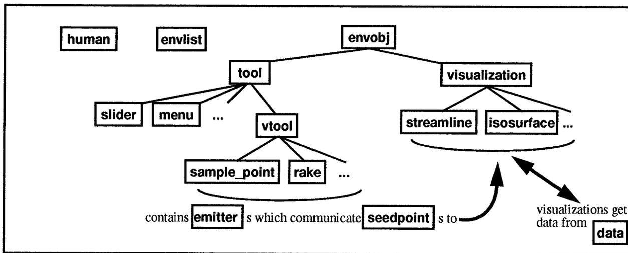
**Fig. 3** The object hierarchy of the virtual windtunnel. `sample_point` and `rake` are example subclasses of `vtool`, while `streamline` and `isosurface` are example subclasses of `visualization`. The `envlist` object maintains lists of the `envobj`s in the environment, and the `human` object manipulates objects through the `envlist`.
