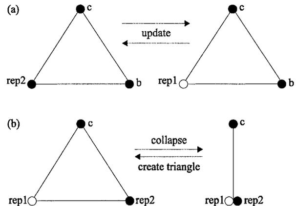
**Figure 2: Two events in the triangle database during clustering are of interest for the reconstruction of the original triangles: Collapsing triangles (a), and triangles whose vertices are updated (b).**
