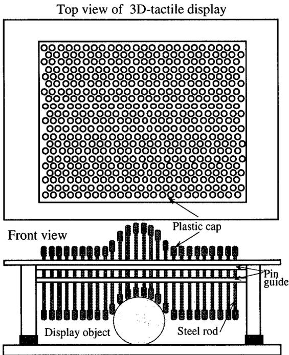
**Fig. 1 Structure of the 3-dimensional tactile display.** Area of displayed surface:125mm<sup>2</sup>, Pin pitch: 2mm, 3mm and 5mm. Zigzag pin arrangement.
