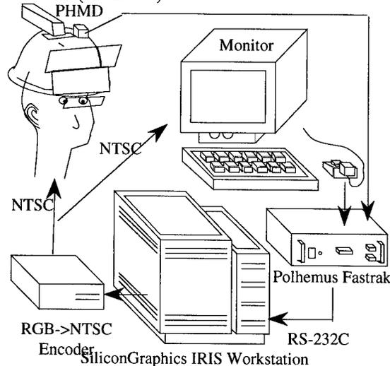
**Figure 9. Prototype System for Fused Environment**
