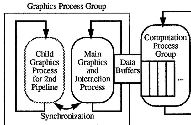
**Fig. 4** The computational processes of the virtual windtunnel, including the optional child graphics process created when there is a second graphics pipeline used for stereoscopic display. The computation process creates several parallel sub-processes that call the compute functions of the environment objects.
