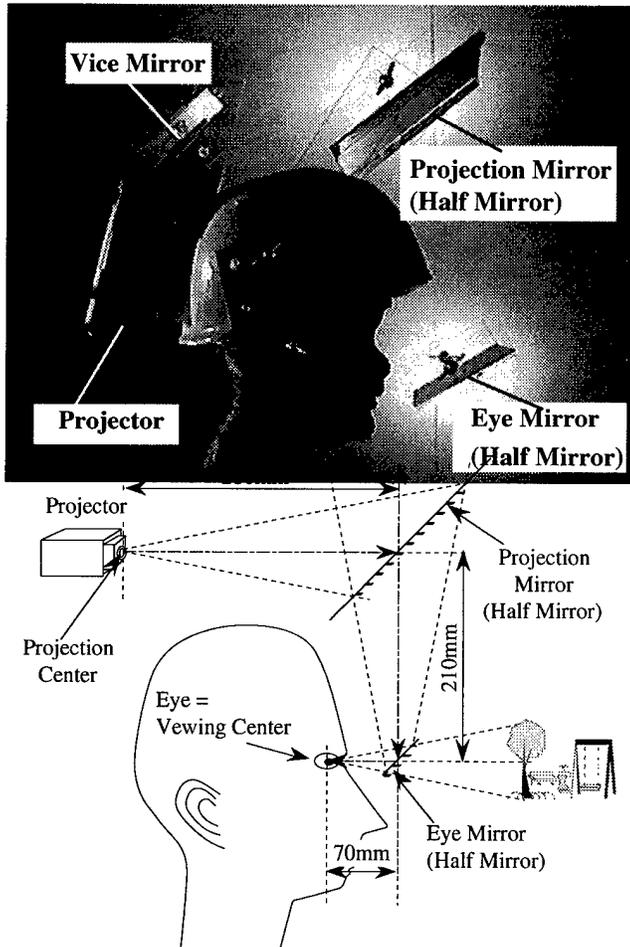
**Figure 8. PHMD: Appearance, Optical Structure**
