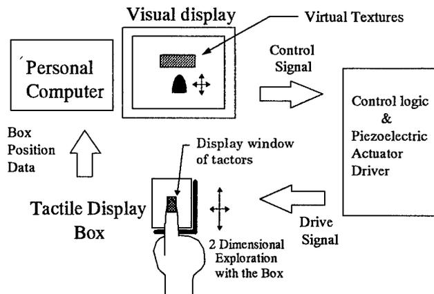
Fig. 1 Schematic of a vibratory tactile display
