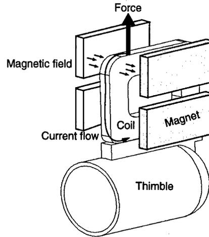
**FIGURE 3. Electromagnetic force generation for finger coil thimble.**
