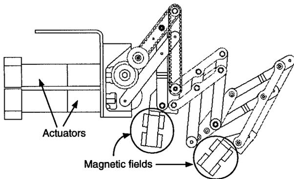
**FIGURE 4. Electro-magnetic interface attached to the ISU exoskeleton.**
