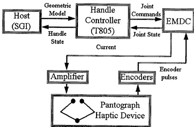
Figure 4. System Connections
