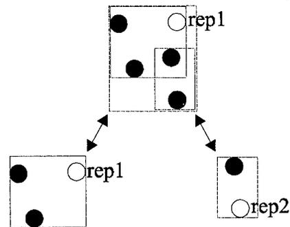
**Figure 3: During the clustering, two vertex clusters are joined into one, and the effect on the triangles is recorded. The inverse operation, cluster expansion, uses the recorded data to reconstruct the triangles.**
