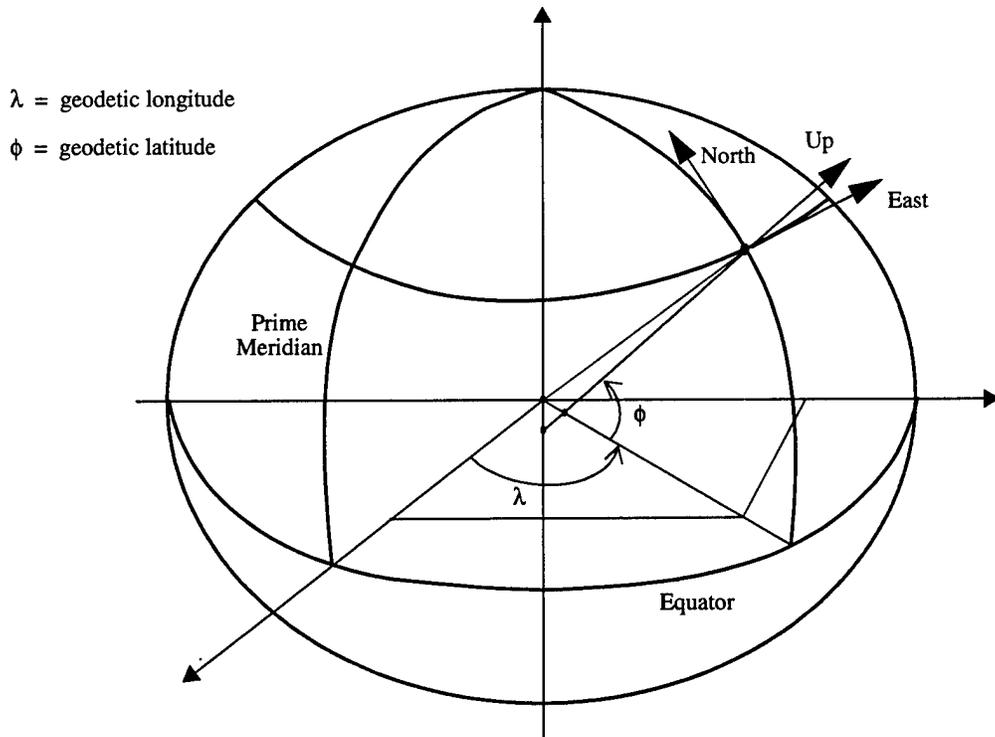
FIGURE 2-1. STABILIZED FRAME (EAST, NORTH, UP) AT A PARTICULAR POINT ON THE EARTH
