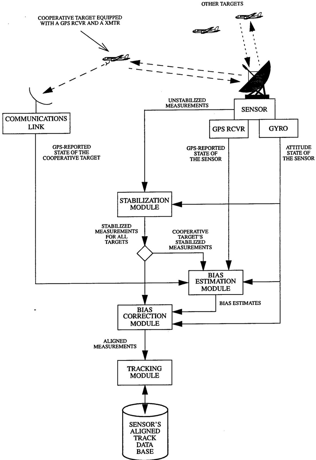
FIGURE 3-2. MEASUREMENT-ALIGNMENT ARCHITECTURE
