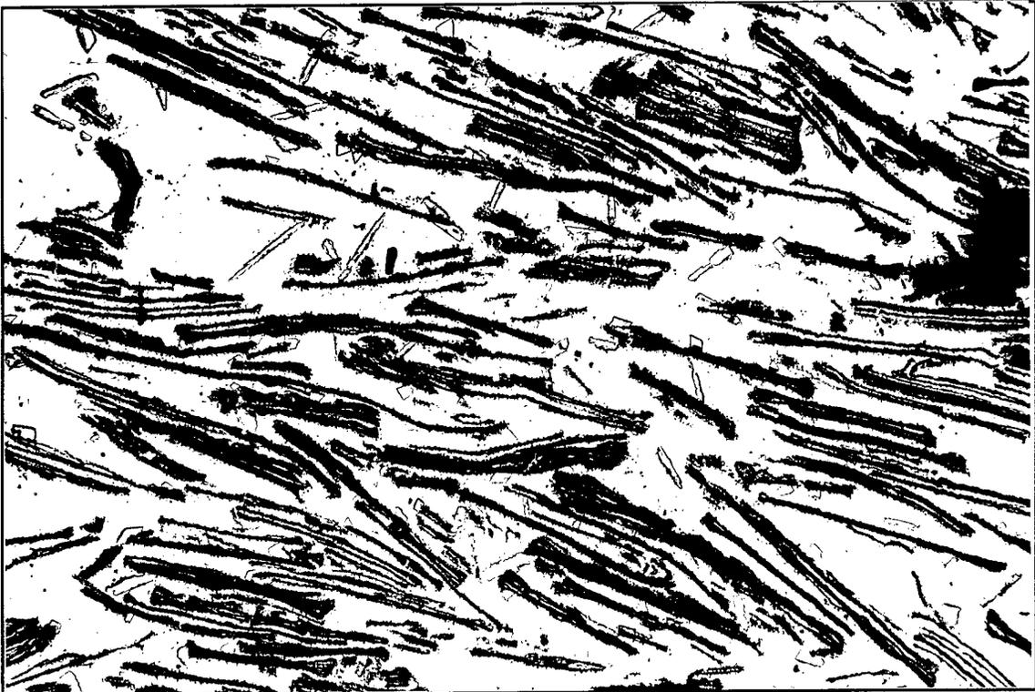
**Figure 14-** Microstructure of Al/Gr Composite (Sample D). Less Reaction with Flake Resulted in Higher Thermal Conductivity and Lower CTE. (Scale: 1cm = 80 $\mu$ m).
