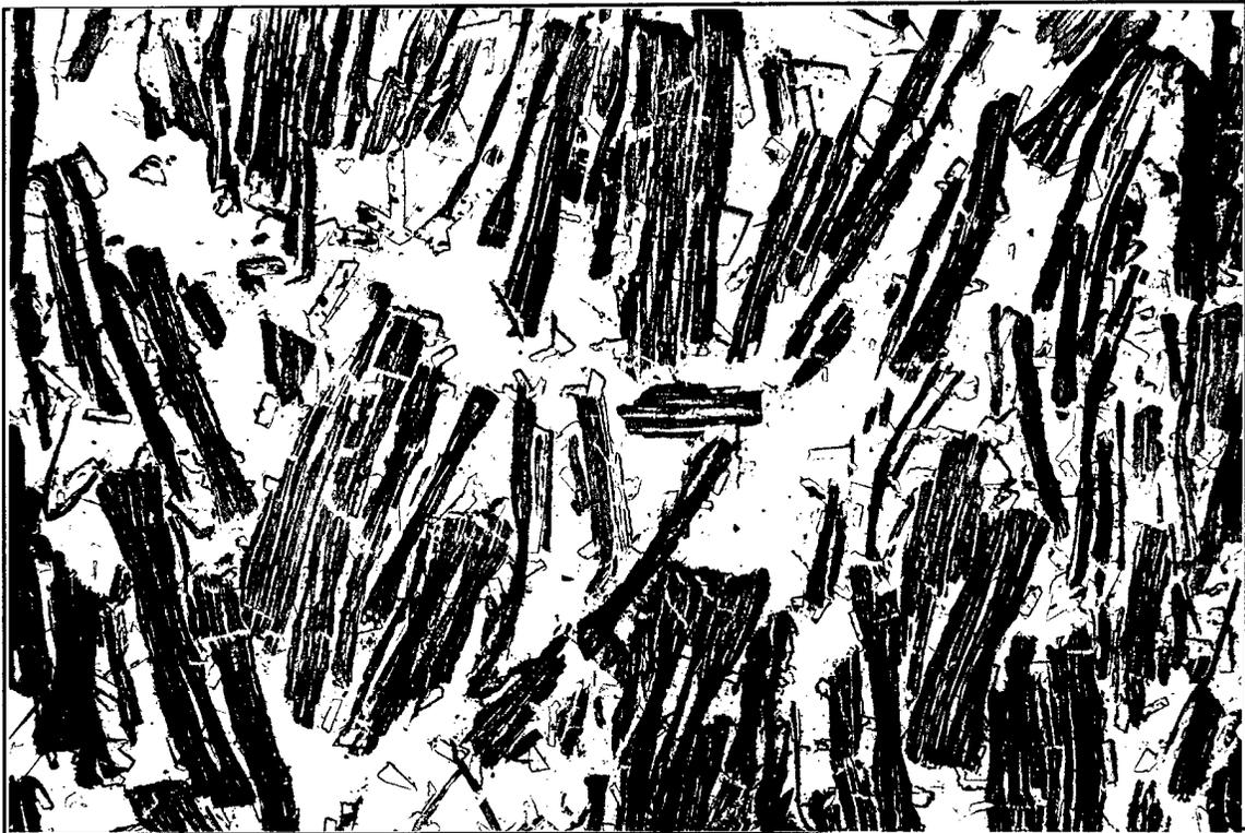
**Figure 13-** Micrograph of Al/Gr Composite (Sample B). Significant Flake Reaction Occurred Because of Defective Molybdenum Coating. (Scale: 1cm = 40 $\mu$ m)
