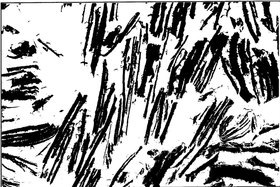
**Figure 12-** Composite Containing Molybdenum-Coated Graphite Flake in 443 Alloy Matrix. Protective Molybdenum-Coating Prevented Graphite Flake Reaction with Matrix. (Scale: 1 cm = 40 $\mu$ m).
