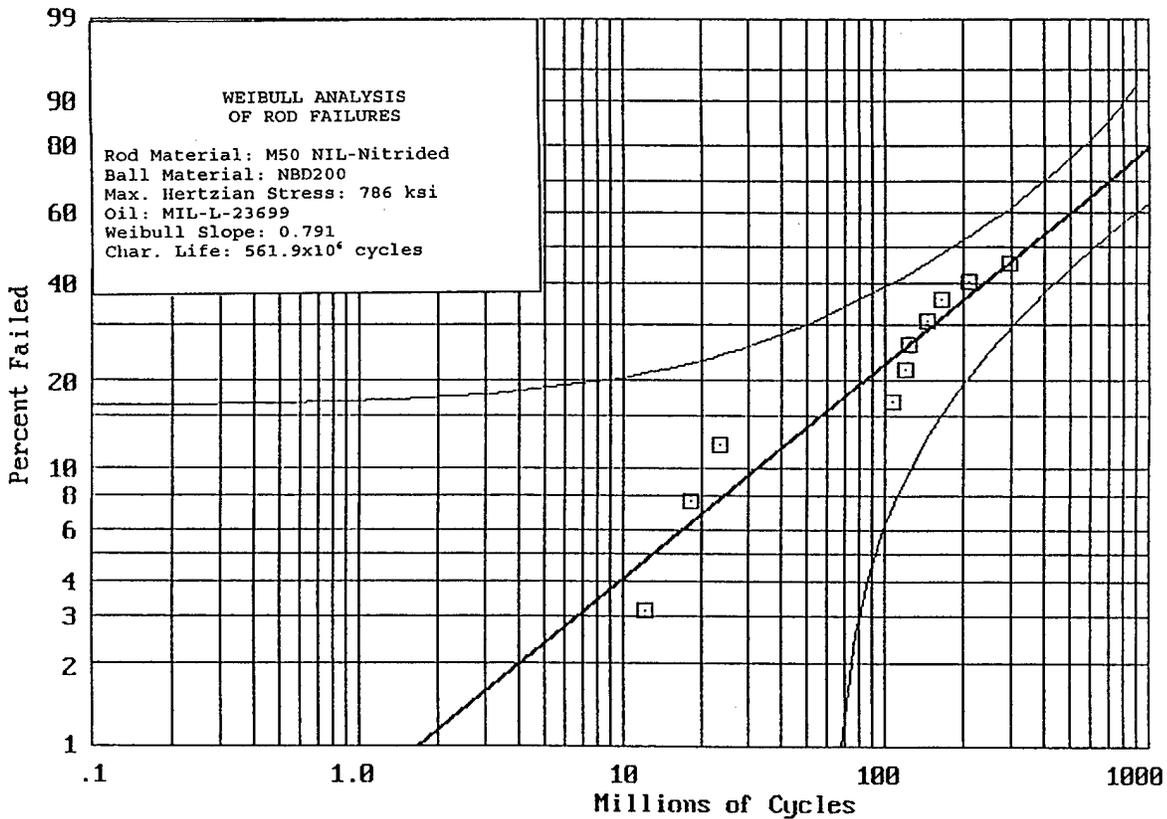
Figure 3 Weibull analysis of rod failures, 561.9 million cycles.
