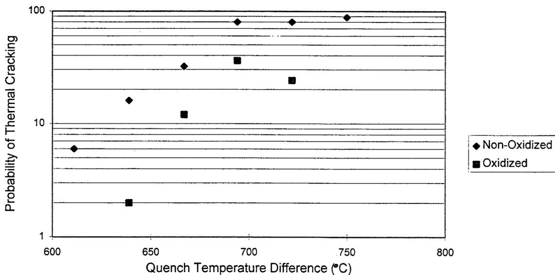
Figure 1 Weibull comparison: oxidized vs non-oxidized balls.
