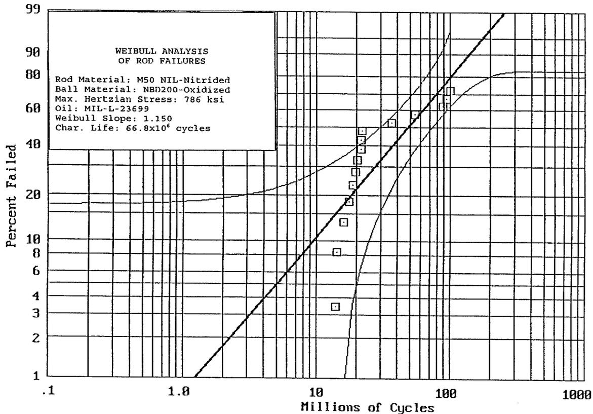
Figure 4 Weibull analysis of rod failures, 66.8 million cycles.
