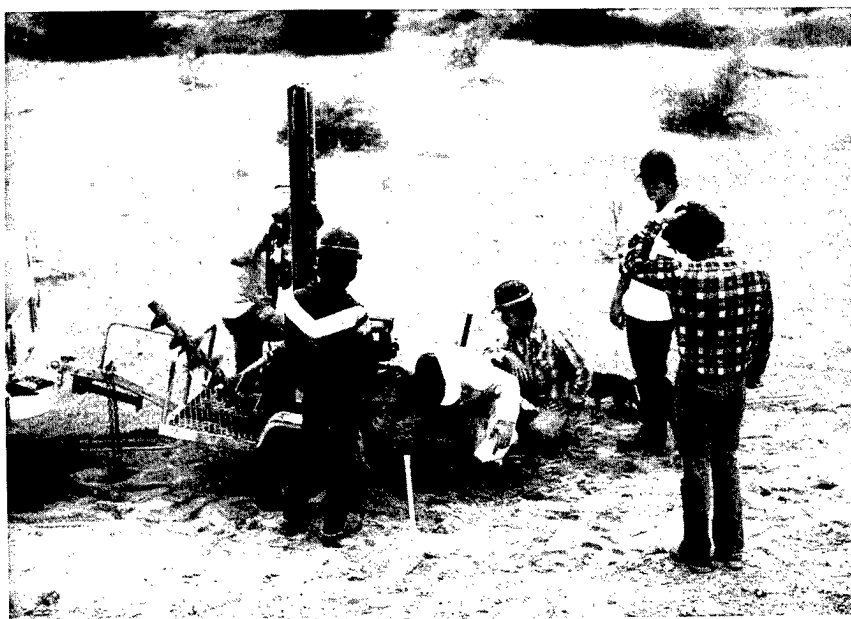
Figure 38. Augering holes to the water table and collecting soil, water, and salinity data are all essential steps in determining the growth potential of native riparian trees and shrubs. Photo by J. Disano.
