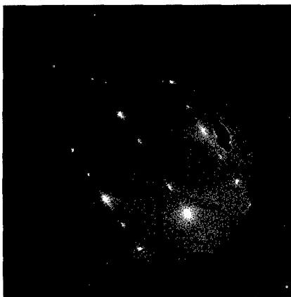
Fig. 3 A LEED pattern of the homoepitaxial (001) film exhibiting 2\times 1 single-domain surface structure. The electron energy is 170 eV.
