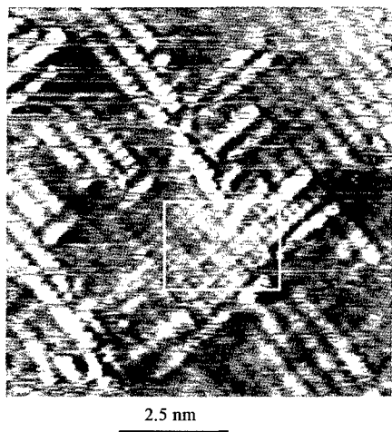
Fig. 4 A high resolution STM image of the diamond (001) film showing local 1x1 structure ( sample bias: 800 mV; tunneling current: 0.5 nA).
