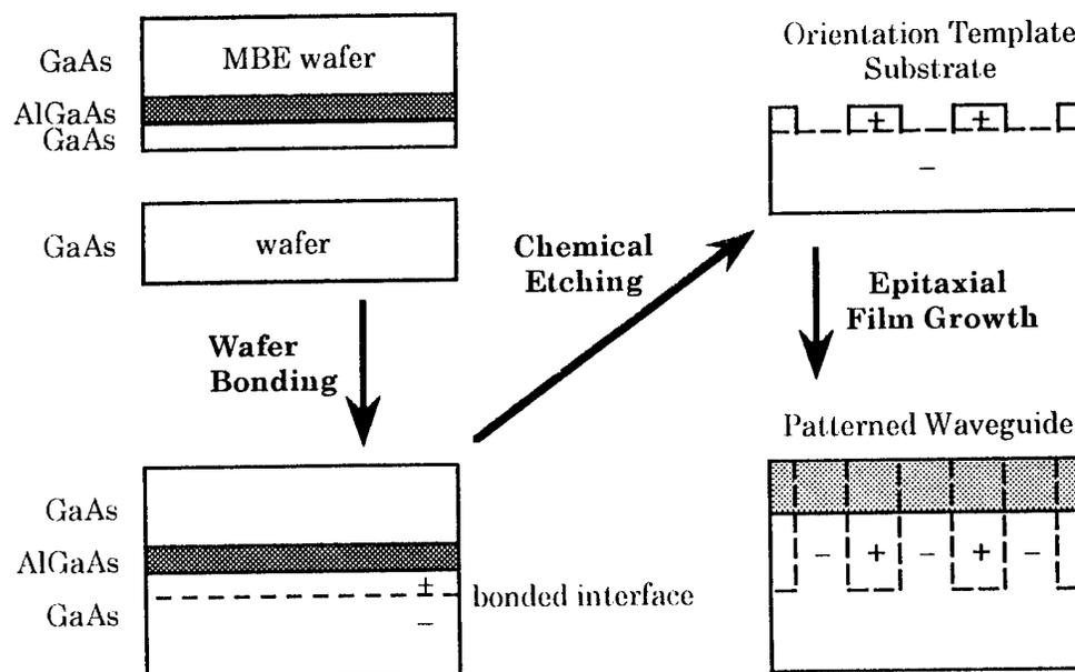
Figure 1: Fabrication process for orientation template substrate and nonlinear grating waveguide.
