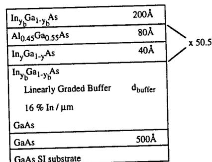
FIG. 1. Layer structure for  $\text{In}_y\text{Ga}_{1-y}\text{As}/\text{AlGaAs}$  square MQWs with graded InGaAs buffer for (a)  $y=0.3$  sample:  $y_b=0.11$ ,  $d_{\text{buffer}}=6000$  Å and (b)  $y=0.5$  sample:  $y_b=0.17$ ,  $d_{\text{buffer}}=10\,000$  Å.
