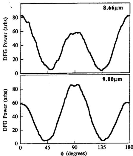
FIG. 3. DFG power vs azimuthal angle  $\phi$  of the sample at output wavelengths of 8.66 and 9.00  $\mu\text{m}$  showing opposite signs of asymmetry due to a sign reversal of the bulk GaAs contribution.
