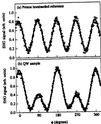
FIG. 4. Measured (hollow circles) and theoretically fitted (solid lines) normalized SHG power vs rotation angle  $\phi$  for the proton bombarded reference (top graph) and QW sample (bottom graph) at a pump wavelength of 4.0  $\mu\text{m}$ .
