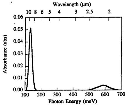
FIG. 1. Intersubband absorption spectrum of the asymmetric coupled QW sample showing peaks at 9.3 and 2.1  $\mu\text{m}$  corresponding to the 1-2 and 1-3 transitions.
