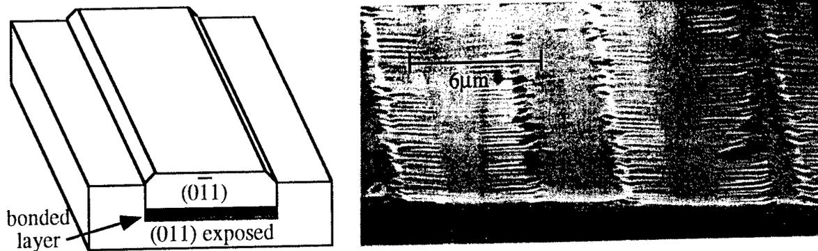
Figure 2: Schematic and SEM micrograph of cleaved cross-section of orientation modulated thin film on orientation template substrate. ( $0.5\mu\text{m GaAs}$ :  $0.1\mu\text{m AlAs}$ :  $0.5\mu\text{m GaAs}$ )
