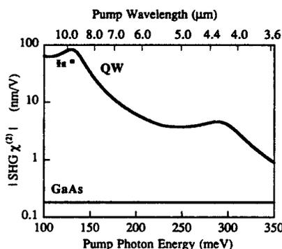
FIG. 2. Measured (points) and theoretical (solid curve) SHG  $\chi^{(2)}$ .
