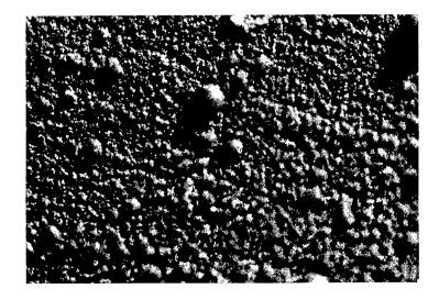
Fig. 4. Microphotograph of the surface of the electrochemically deposited ZrB2 on glassy carbon ( $\times$ 30).
