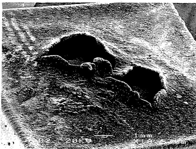
Figure 7 Electrode failure - Rupture (15mm x 15mm SL 'tablet' electrode)
