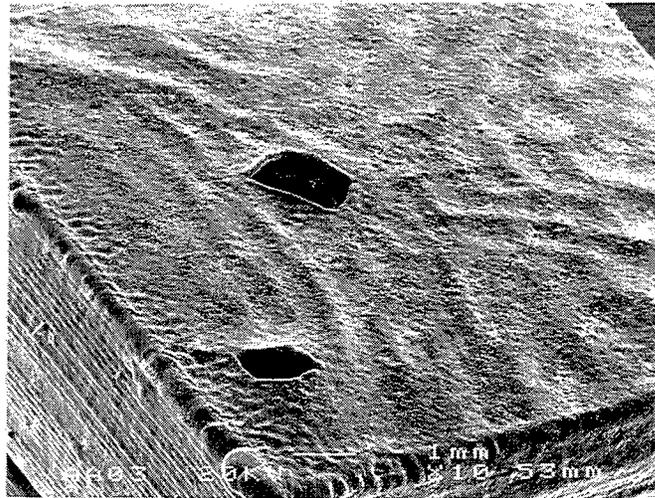
Figure 4 Electrode failure - Peppering (15mm x 15mm SL 'tablet' electrode)
