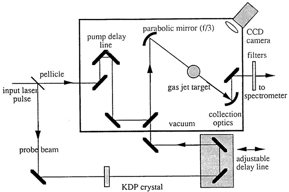
[Fig. 1] Schematic of Thomson scattering experimental setup.
