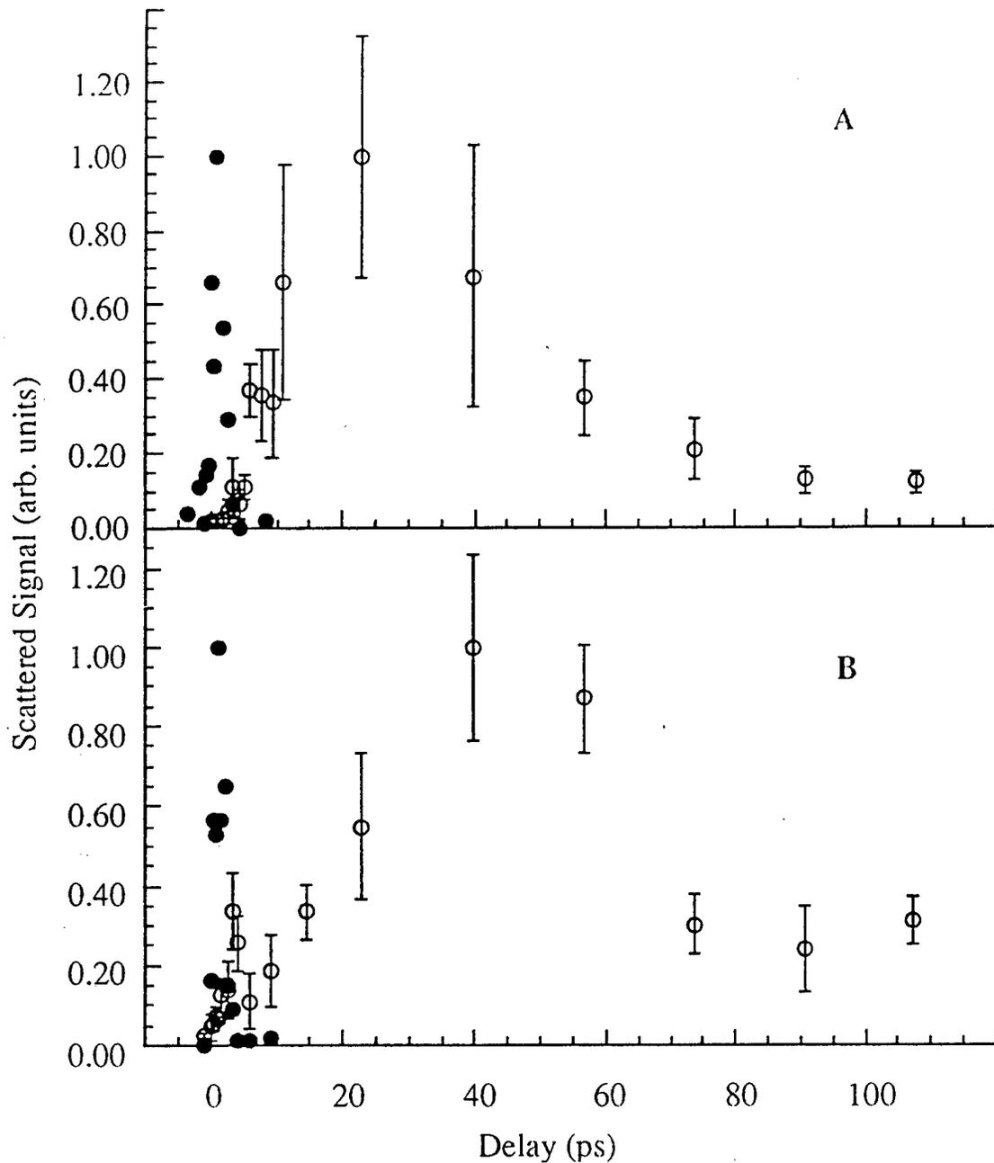
[Fig. 4] Evolution of Thomson scattered spectrum at  $30^\circ$  scattering angle w.r.t. pump laser but  $20^\circ$  w.r.t. the probe: A) hydrogen, B) helium. Open circles are normalized values of the central peak in the scattered spectrum and closed circles are the normalized value of the first order Stokes satellite.
