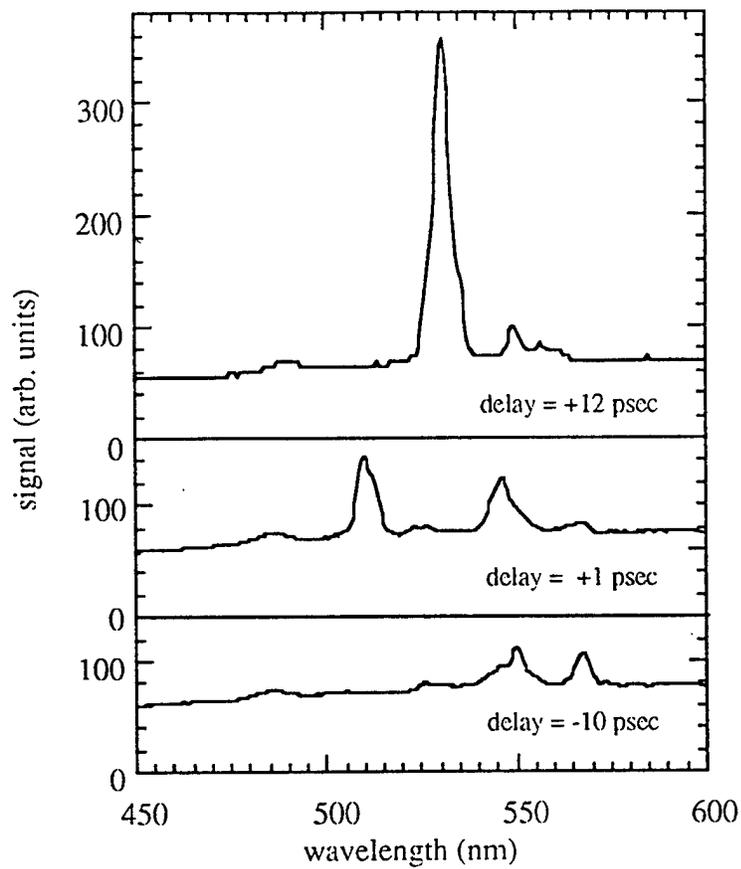
[Fig. 3] Evolution of Thomson scattered spectrum at  $30^\circ$  scattering angle w.r.t. pump laser axis (Pump and probe laser are collinear) for different delay settings between pump and probe pulses. Negative delay implies emission from pump laser alone.
