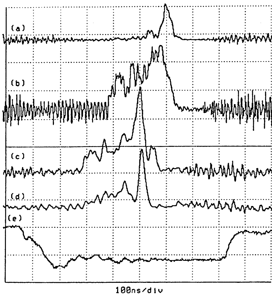
Fig. 4. MELBA experimental shot at 2.2kGauss for the small-orbit gyrotron. (a) signal from 2.5-3.0GHz microstrip filter with peak power corresponding to \sim 0.4\text{MW} . (b) signal from 3.0-3.5 GHz microstrip filter with peak power \sim 0.2\text{MW} . (c) total power measured from horizontally polarized signal, peak power corresponding to \sim 2\text{MW} . (d) vertically polarized signal, peak corresponds to \sim 0.5\text{MW} . (e) Voltage monitor signal (620 keV/div).
