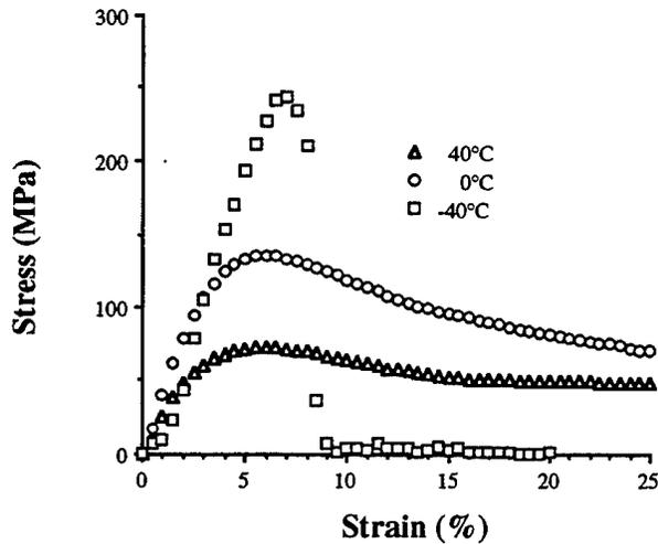
Figure 3. Stress vs. Strain Curves for M30 Propellant
