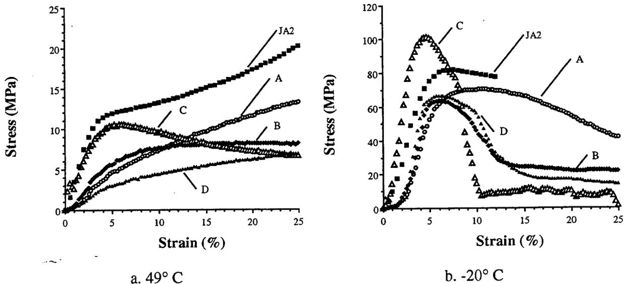
Figure 10. Mechanical Response Curves of Advanced Propellant Formulations Compared to Conventional JA2 Propellant
