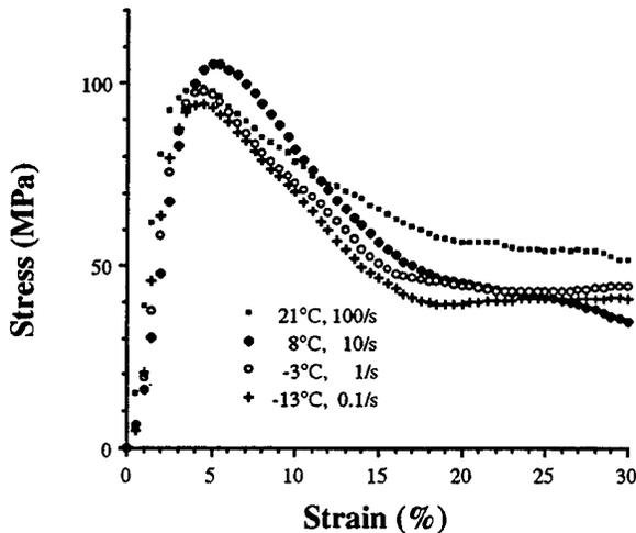
Figure 8. Mechanical Response of M43 at Equivalent Time-Temperature Conditions
