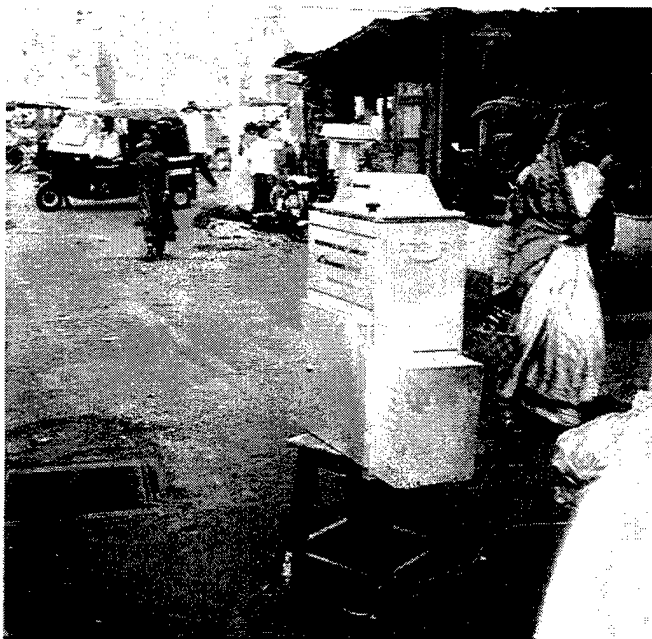
Figure 11. Particle Collector Site in Pune City; Particles up to 10um Diameter Can Be Collected.
