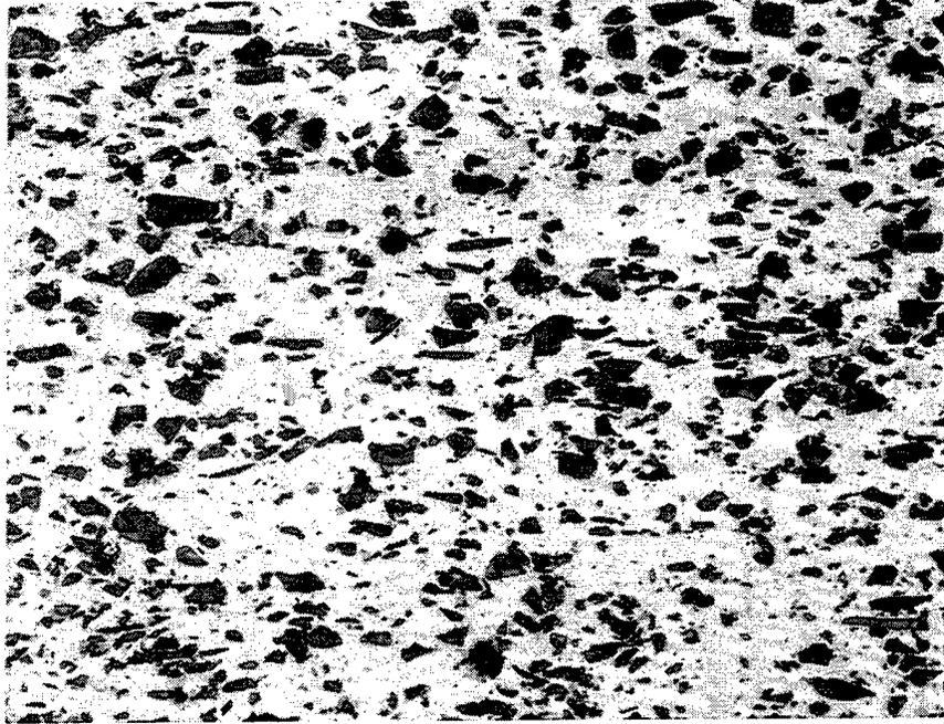
Figure 25: T6 matrix far removed from failure. 320X.
