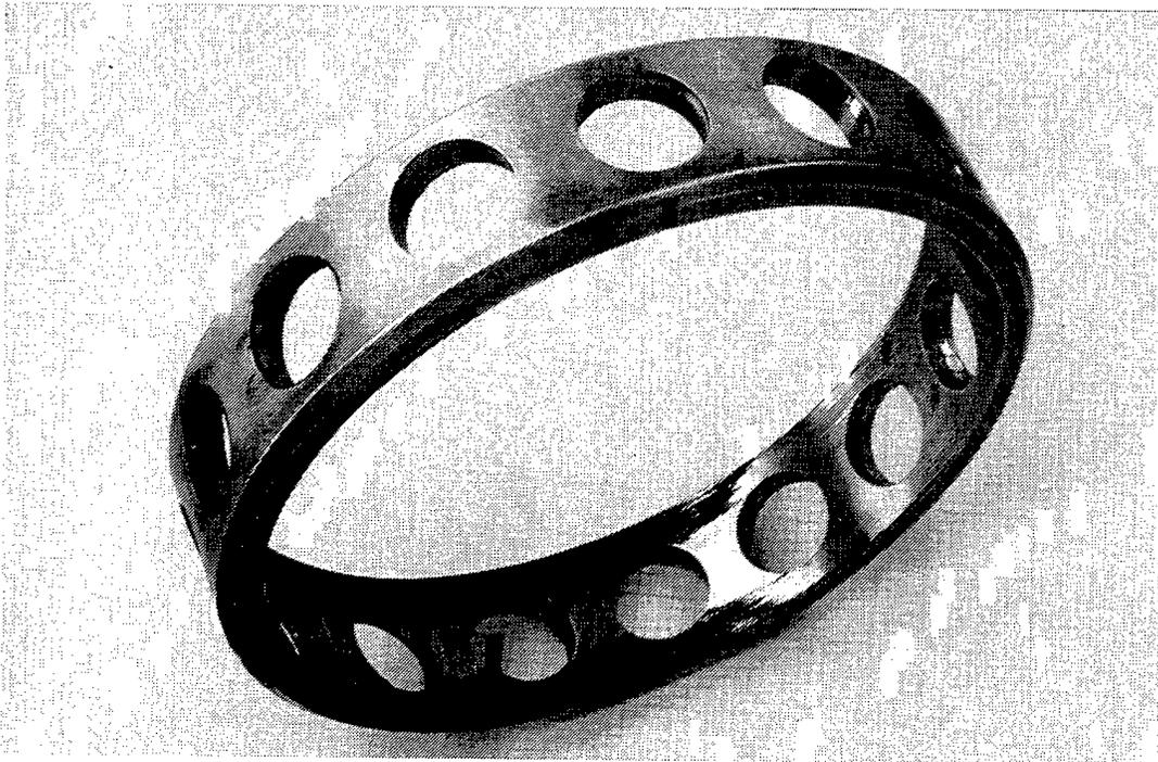
**Figure 56. Cage from Bearing P04** *The severe rub on the inner ring may be due to large vibrations caused by the balls passing over the lube slots.*
