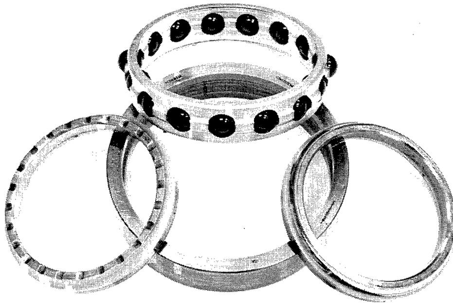
**Figure 46. Hybrid Bearing with Silicon Nitride Balls After Completion of Test Points 37 Through 72**
