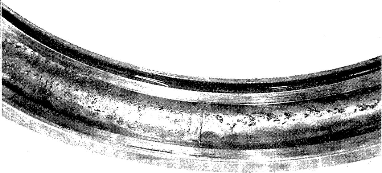
**Figure 20. Spalled Outer Race** *The spall initiated at the EDM notch and wrapped around 360° to join back up with the initiation point. This is a strong indication of the severity of the test and the amount of bearing steel that was liberated before final failure occurred.*
