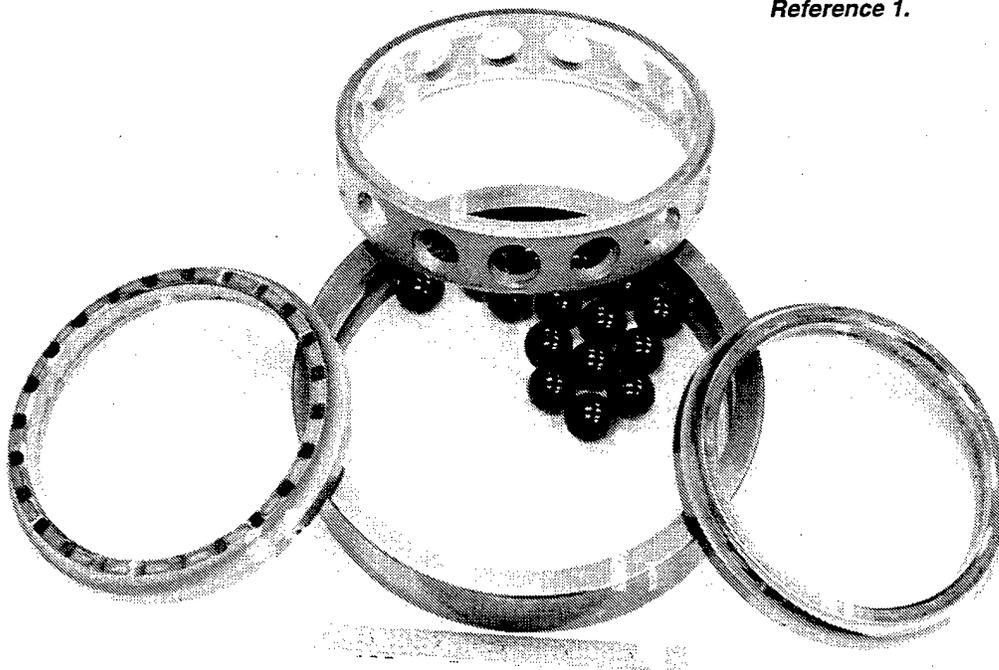
**Figure 53. Hybrid Bearing with Silicon Nitride Balls (P05) After Completion of Test Points 91 Through 101** *Except for scuff marks on the cage, the bearing is in good condition. The absence of discoloration indicates low heat generation.*
