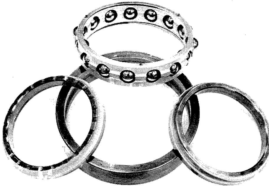
**Figure 42. All-Steel 120-mm Bore Bearing After Completion of 36 Test Points** *Other than a slight rubbing of the cage, this bearing is in good condition. Note that the ball path and the lands of the bearing were nodular thin dense chrome (TDC) plated.*
