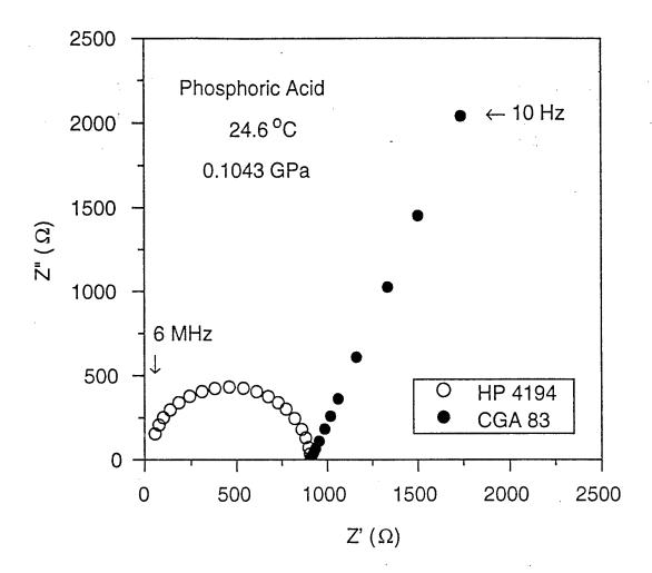
Figure 1. Complex impedance diagram at 24.6°C for 85% phosphoric acid. The solid circles represent data from the Hewlett Packard 4194 and the open circles are data obtained from a CGA-83 Capacitance bridge. The frequencies increase from right to left.
