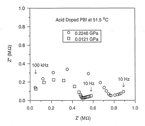
Figure 2. Complex impedance diagrams at 51.5°C and two pressures for acid doped PBI. The open circles (0.2246 GPa) and open squares (0.0121 GPa) represent datum points obtained using a CGA-83 Capacitance bridge. The frequencies increase from right to left and the frequency range is 10 to 10<sup>5</sup> Hz.
