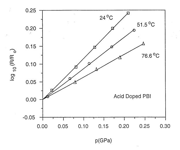
Figure 3. Relative electrical resistance vs. pressure at various temperatures for acid doped PBI. Also shown are the best-fit straight lines.
