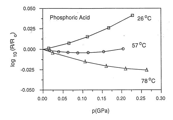
Figure 4. Relative electrical resistance vs. pressure at various temperatures for 85% phosphoric acid. Also shown are the best-fit quadratic equations.
