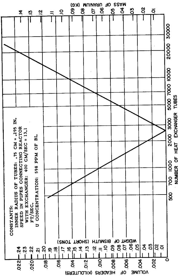
Figure 24c. Mass of uranium in and volume of headers v number of tubes.
