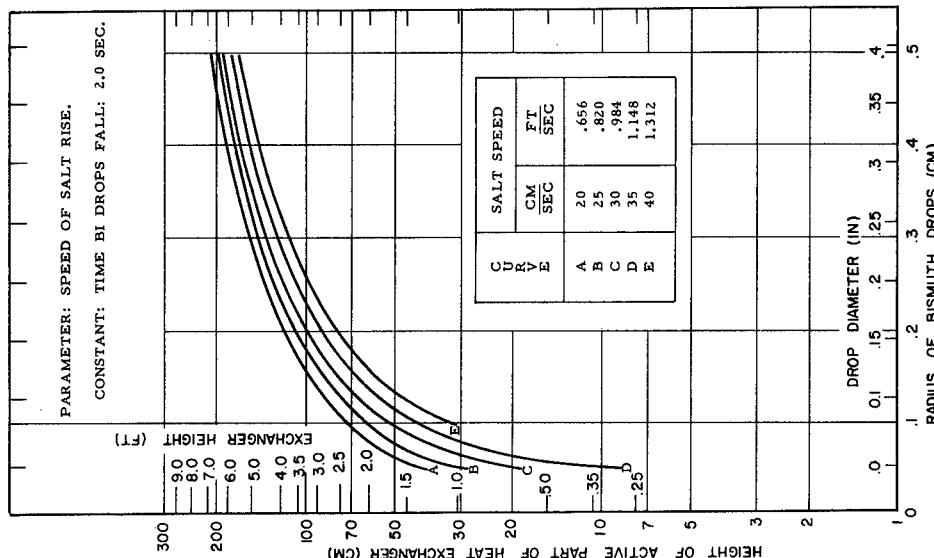
Figure 27a. Height of active part of heat exchanger vs time bismuth drops fall.
