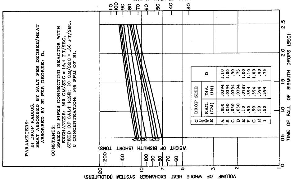
Figure 3lf. Mass of uranium in and volume of whole heat exchanger system vs time bismuth drops fall.
