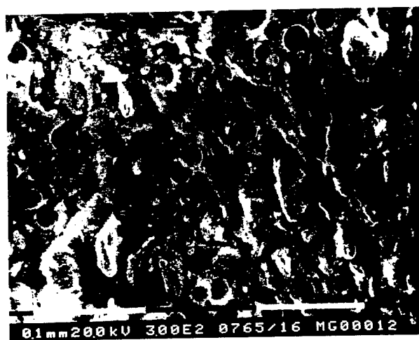
Figure 2. SEM of sintered porous magnetic gel. The circular holes are the locations of the polystyrene beads ( 21.7 \pm 3.2 \mu\text{m} diameter), at a starting volume fraction of 0.015. The voids are the remnants of the polystyrene beads that were thermally removed, while the structure of the gel is maintained.
