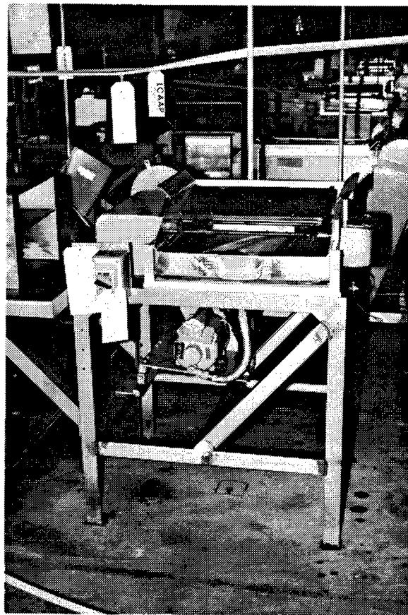
Figure 42. Building 135: Cup - Anvil Shaker for .30 caliber ammunition manufactured by the Emhart Manufacturing V&O Division and received by the plant in 1954.
