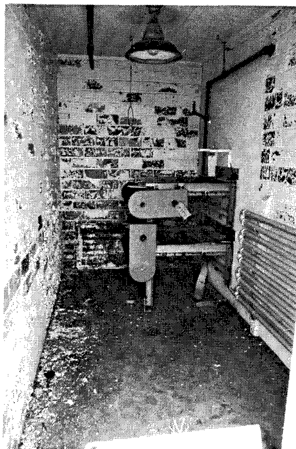
Figure 109. Building 192-B: Dryer Oven in the P.R. Cake Drying House.
