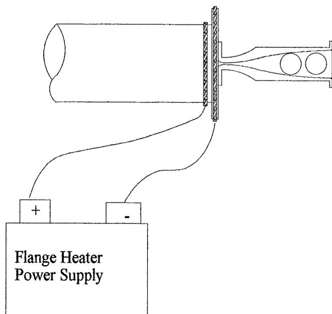
Figure 21 Flange Heater Schematic
