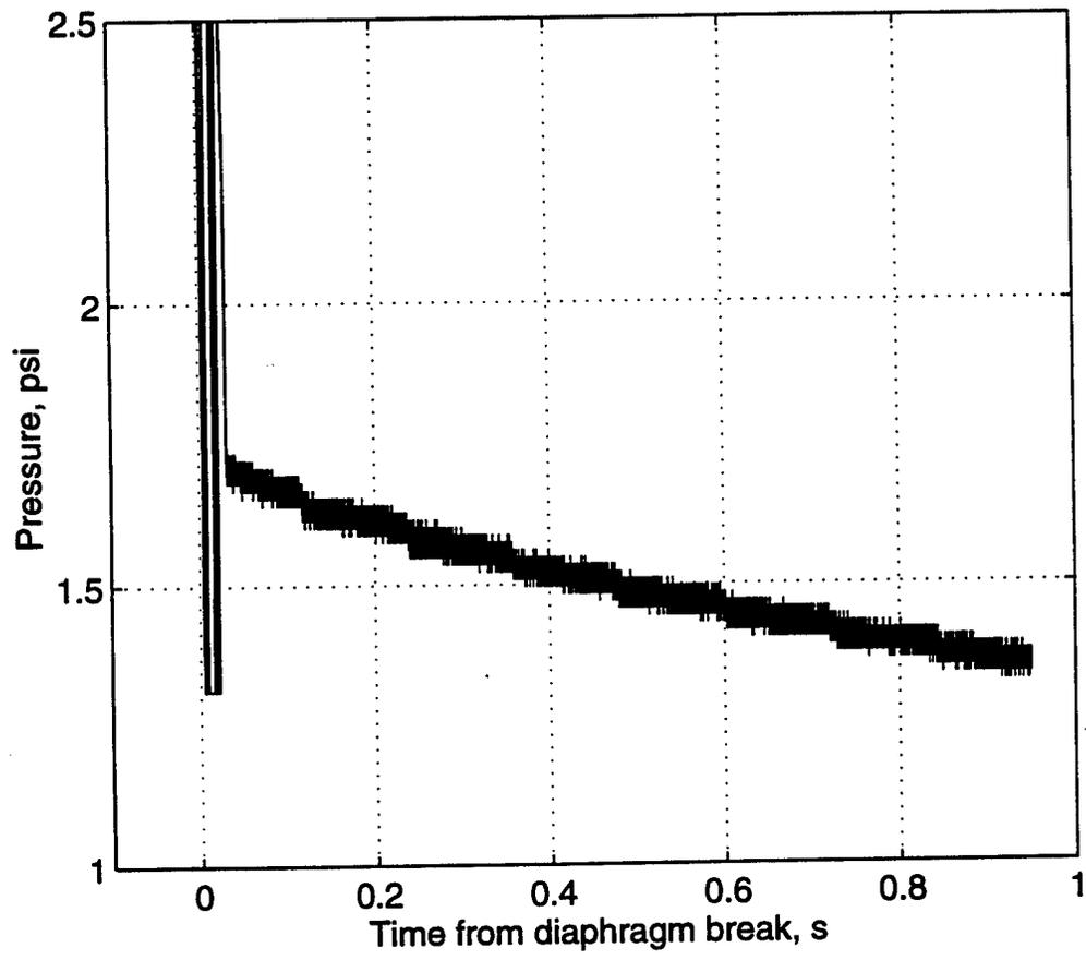
Figure 45 Sample Kulite Pressure Trace
