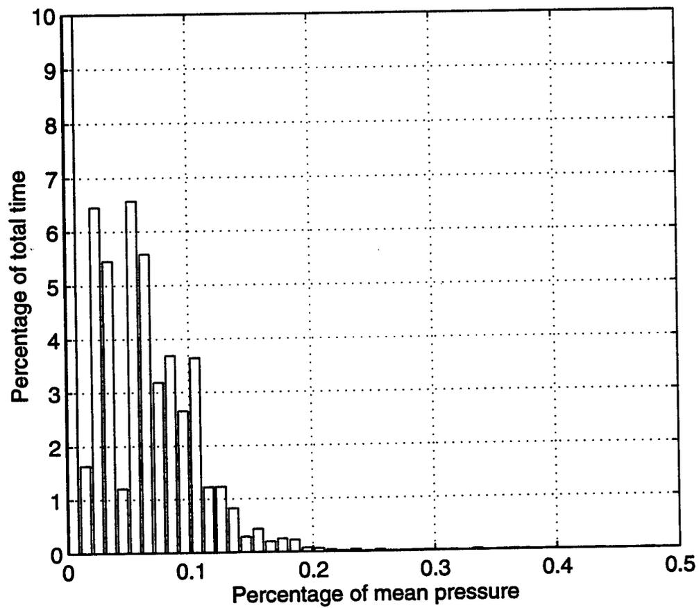
Figure 78 Histogram of Low Noise Segment
