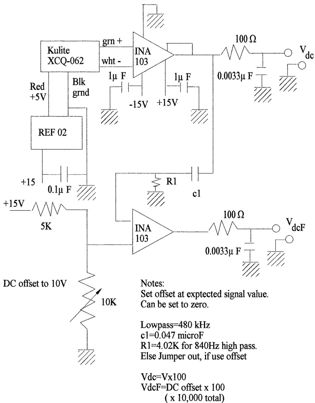
Figure 26 Kulite Amplifier Box Schematic
