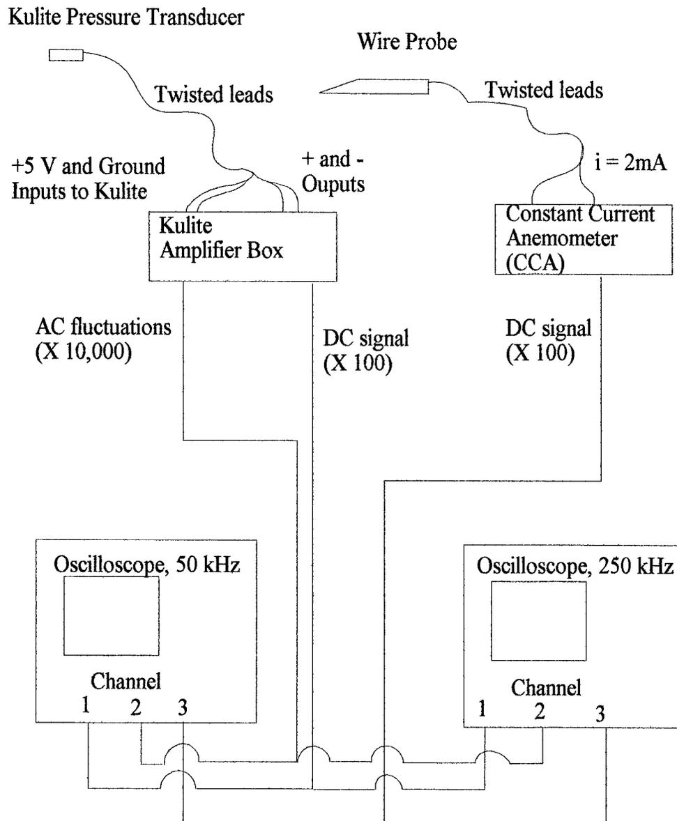
Figure 27 Instrumentation Set-up
