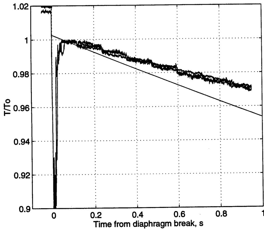
Figure 57 Normalized Temperature Comparison with Theory
