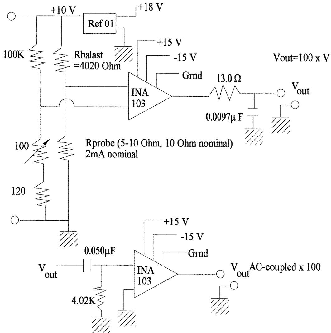
Figure 30 Constant Current Anemometer Schematic
