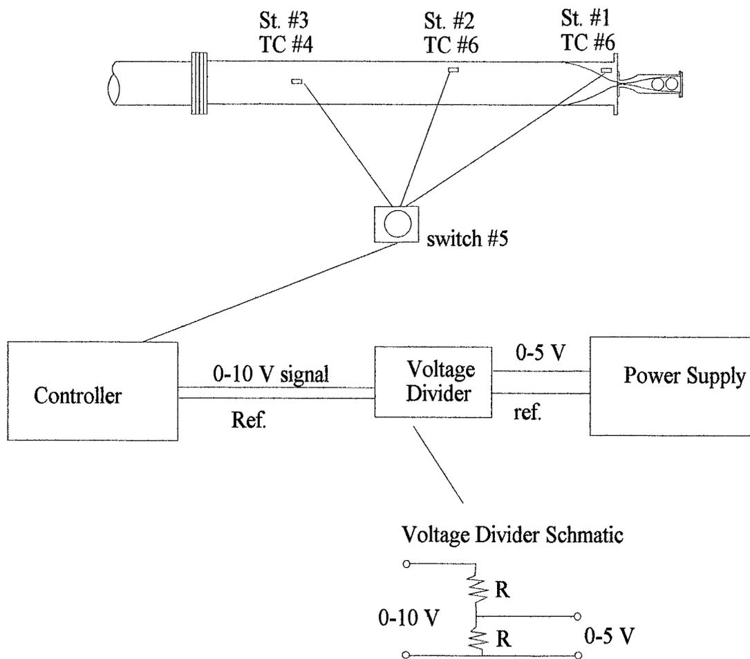
Figure 18 Schematic of Controller Output
