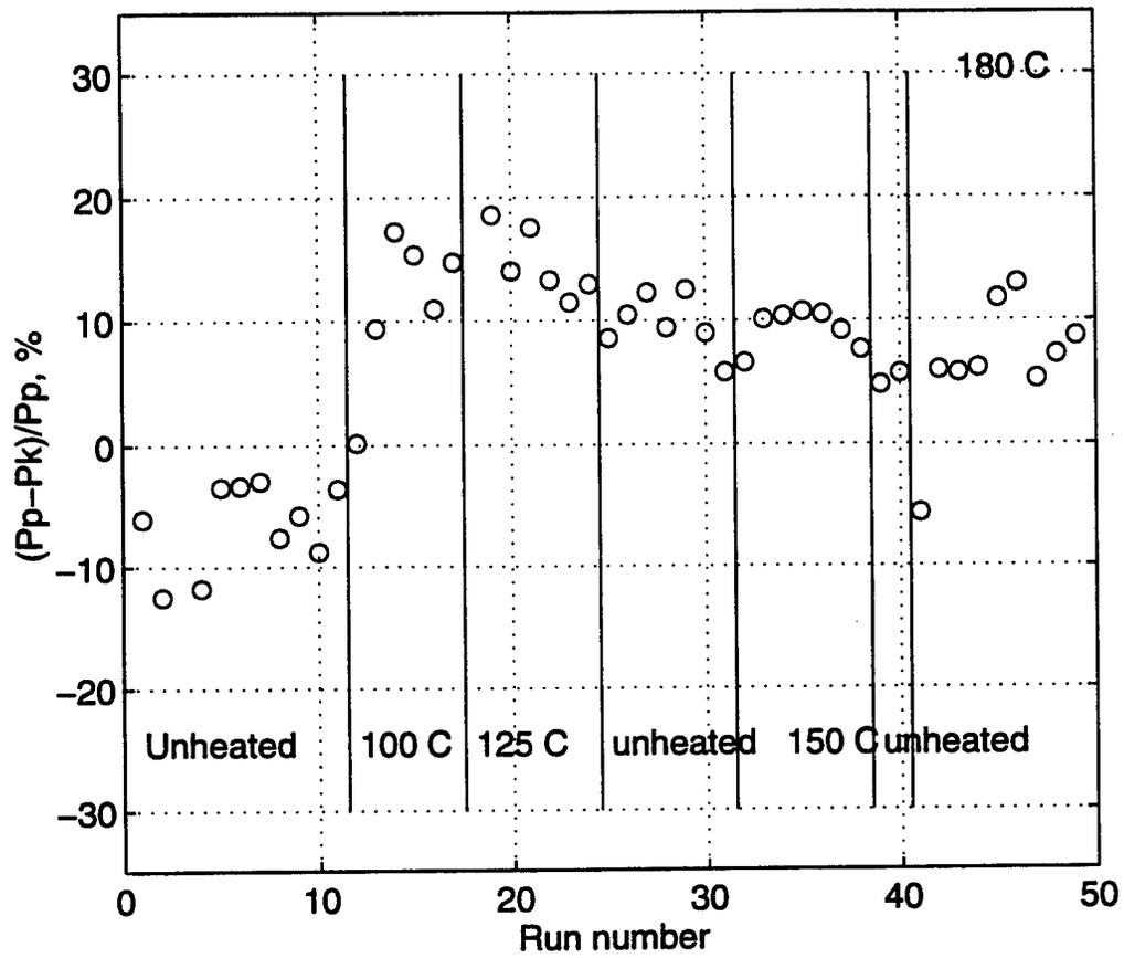
Figure 104 Percent Difference Between Kulite and Paroscientific Pressure Transducers
