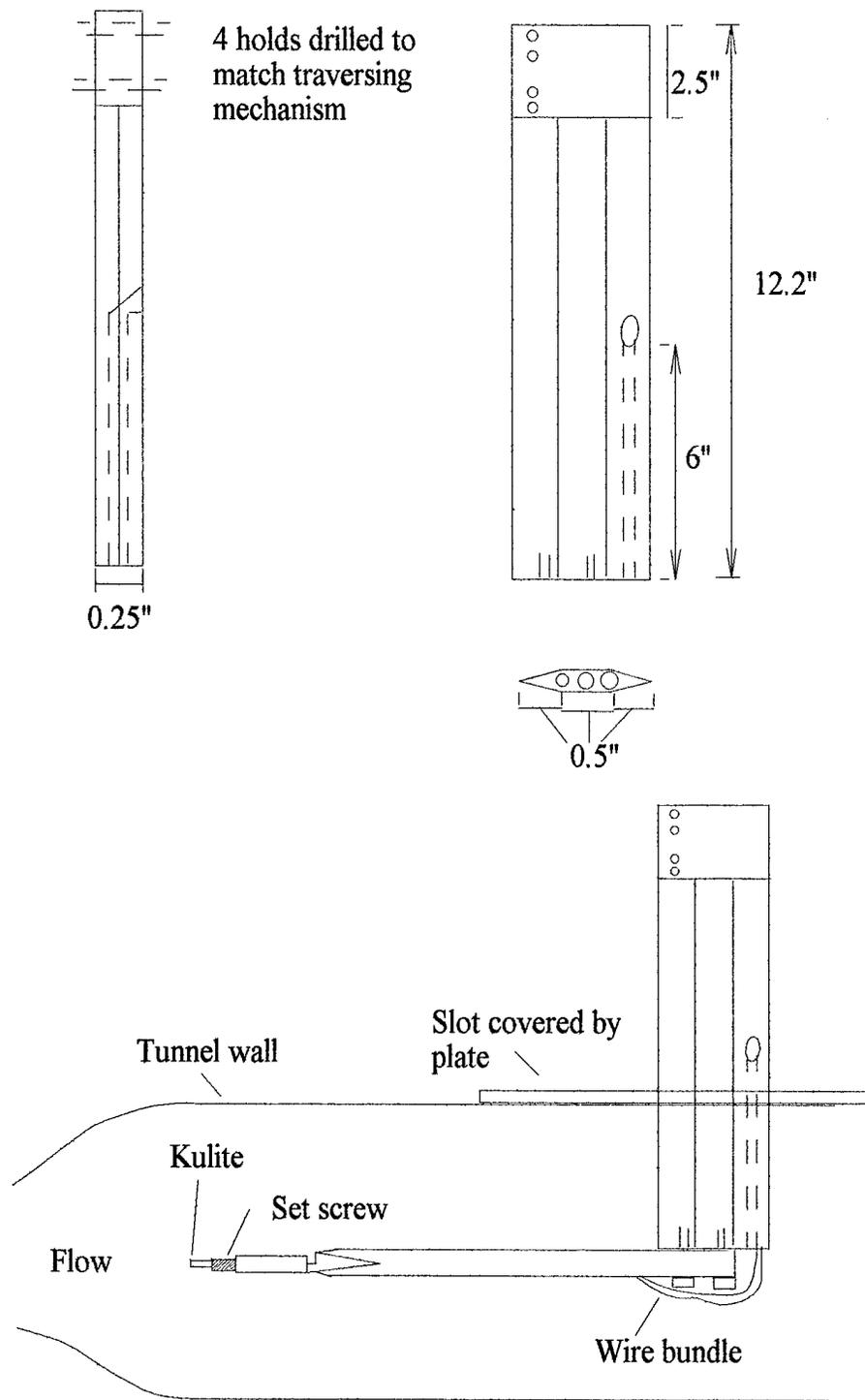
Figure 23 Pressure Rake Traverse and Tunnel Positioning
