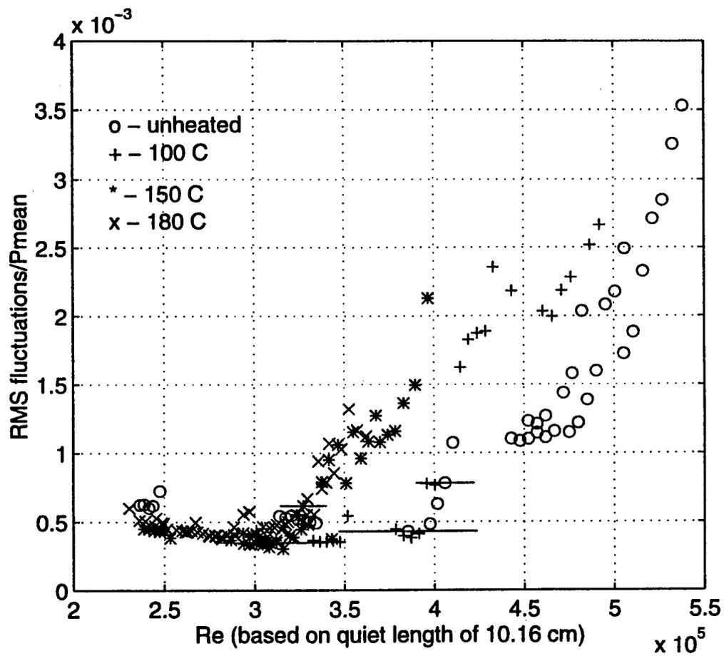
Figure 108 RMS Noise Levels vs. Reynolds Number
