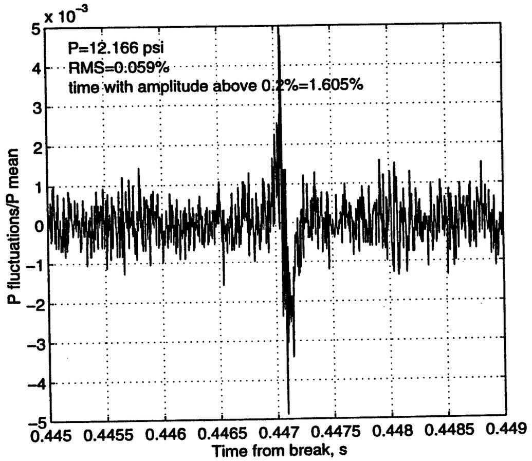
Figure 83 Portion of Slightly Noisy Segment
