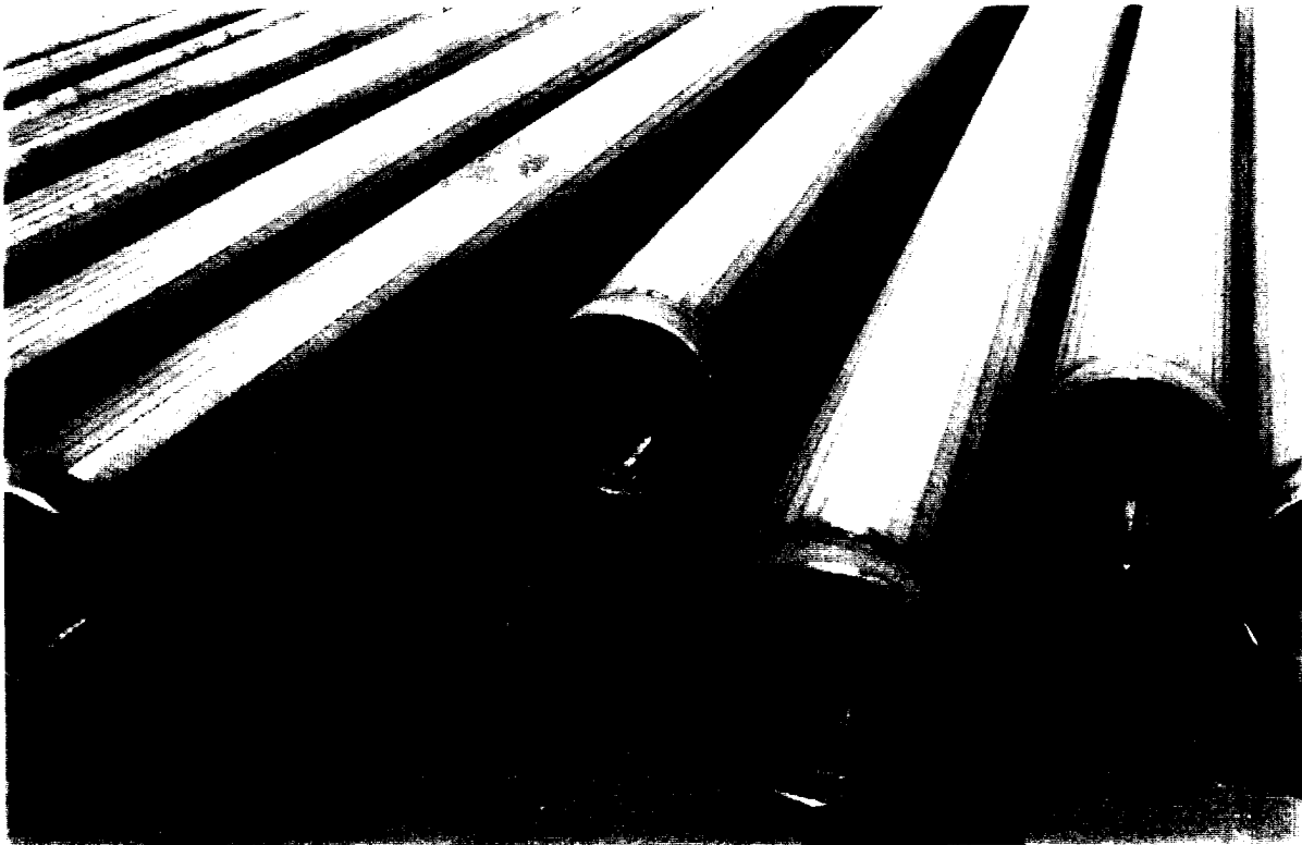
12. Stainless steel well screen used as collector pipes for pressure relief system.
