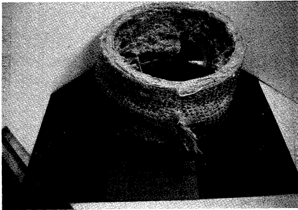
FIGURE 52. POSTTEST PHOTO OF SPIN TEST STRUCTURE 5 SHOWING BLADE EXIT POINT. DISK FRAGMENTS WERE STUCK IN THE RING AFTER THE TEST
