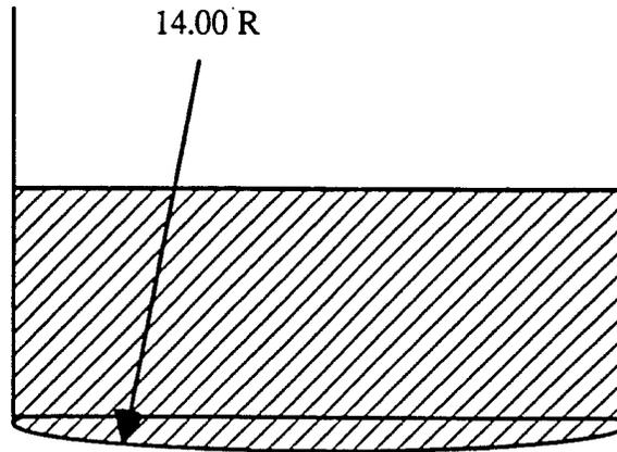
Figure 3 - Cross Section Showing Bearing Face Radius
