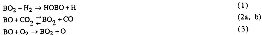
A High-Temperature Fast-Flow Reactor (HTFFR) was used to measure rate coefficients for reaction 1 and upper limits for 2a and 2b. The High-Temperature Photochemistry (HTP) technique was used to obtain an upper limit for 2a, as well as to measure rate coefficients for reaction 3.
