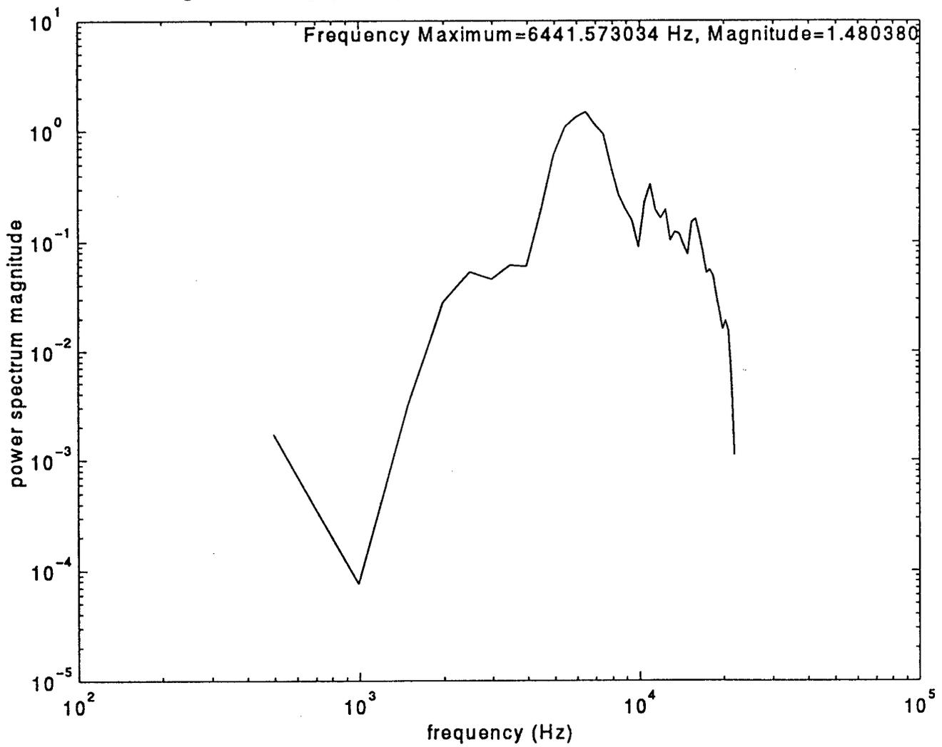
Figure 11: Conditionally sampled high frequency acoustic signal exponentially fitted
