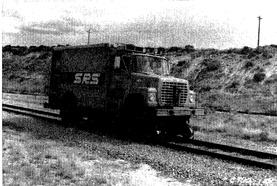
Photo 2. High-rail Internal Rail Defect Vehicle
