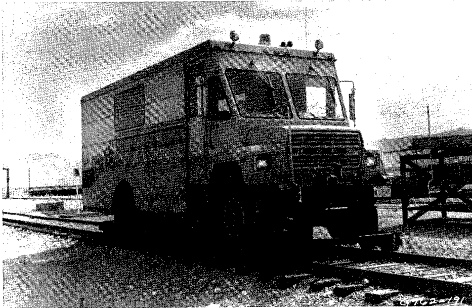
Photo 1. High-rail Track Geometry Vehicle
