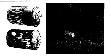
The Skipper mission was a space experiment involving a small satellite (above left) traveling at about 8 km/sec making a controlled re-entry for the purpose of measuring ultraviolet radiation from the shock-heated gas at the nose region. To model the reentry, a concurrent, three-dimensional simulation capability based on the Direct Simulation Monte Carlo (DSMC) method was developed in collaboration with Phillips Laboratory, EAFB.
