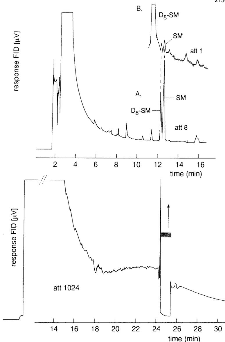
**Figure 3.** Chromatograms of a 400- $\mu$ l on-column injection of a standard solution of SM and D<sub>8</sub>-SM on GLC configuration 2. At the bottom the pre-column chromatogram is shown. The shaded area designates the fraction which was trapped and reinjected onto the analytical column. The top chromatograms show (A) a standard of SM and D<sub>8</sub>-SM and insert (B), concentrations of SM and D<sub>8</sub>-SM near the detection limit.
