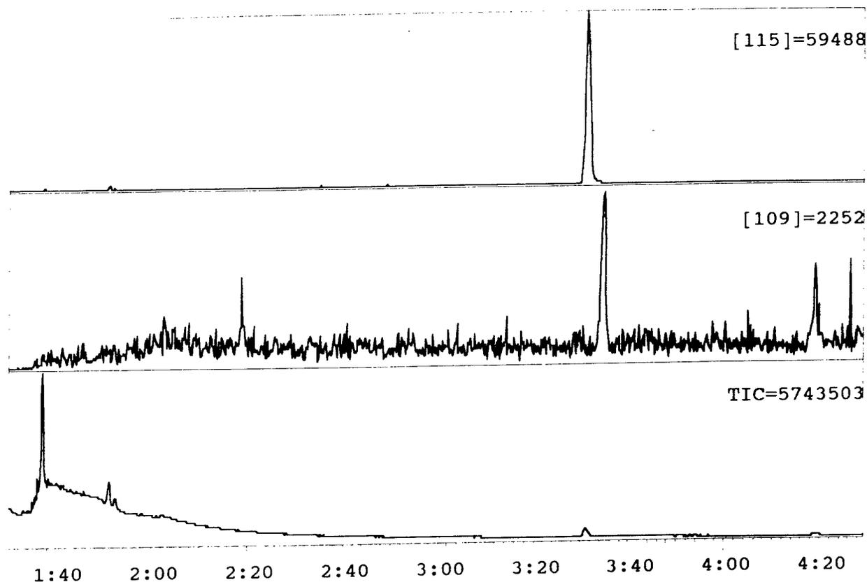
**Figure 6.** GC-MS chromatograms of an ethyl acetate extract of a blood sample drawn from a hairless guinea pig at 40 min after intravenous administration of 8.2 mg SM/kg. The peak detected at  $m/z$  109 (middle chromatogram) is SM (55.7 ng/ml blood), the peak detected at  $m/z$  115 (upper chromatogram) is  $D_8$ -SM (525 ng/ml blood). The lower chromatogram shows the total ion current (TIC).
