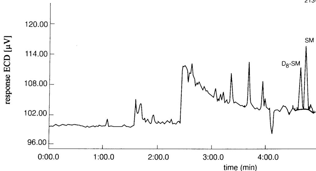
**Figure 4.** Detection of SM and D<sub>8</sub>-SM in a 3-ml extracted blood sample, by on-column injection of 400 µl of ethyl acetate extract on GLC configuration 2. Notice the absence of a solvent peak.
