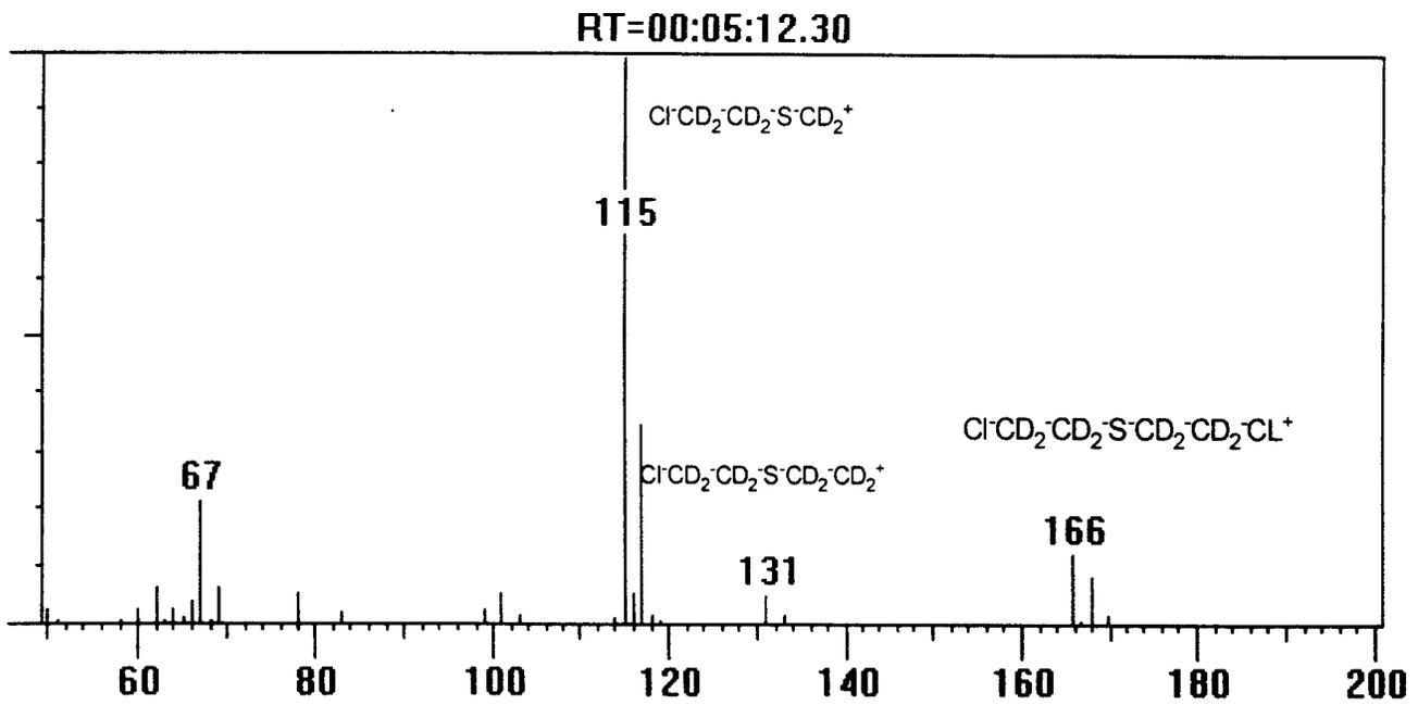
Figure 5. Mass spectra (ei) of (a) sulfur mustard, and (b) D<sub>8</sub>-sulfur mustard.
