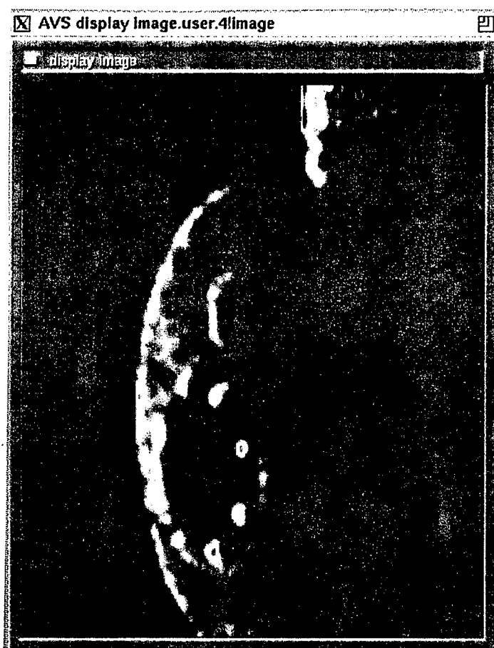
Fig. 7 — Fan-beam image of object B at a 45^\circ angle of incidence. The object is suspended in the water tank.
