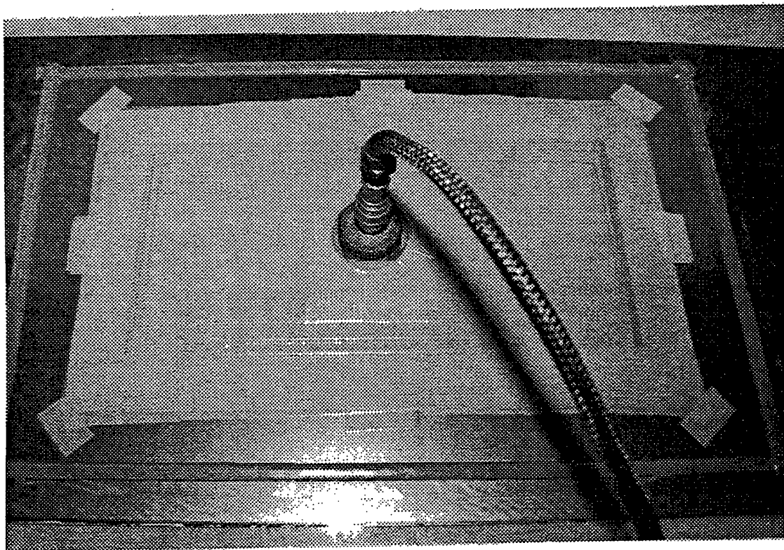
Figure 18. Laboratory Vacuum Molding Trial of NPE 2916.
