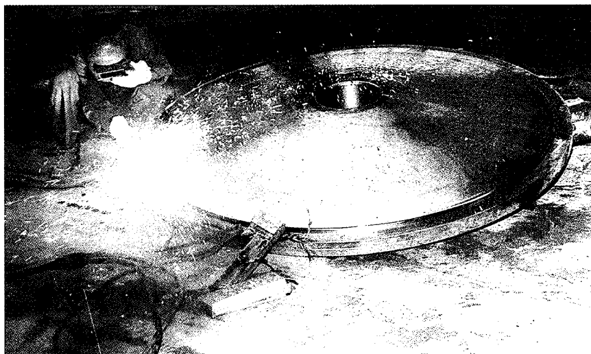
7th U.N. inspection team in Iraq, October 1991: destruction of dies for missile components by electric torch.
