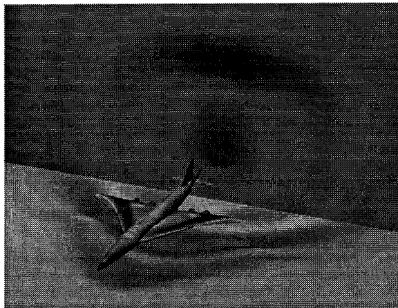
Figure 11: Pressure Contours and Sonic Boom on a Representative HSCT Configuration
