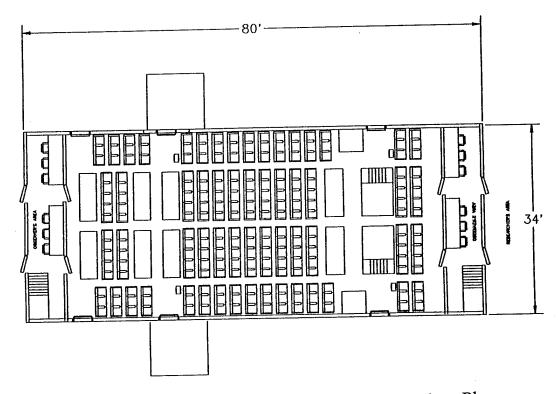
Figure 8 - Mega-Wide Body Main Deck Floor Plan
