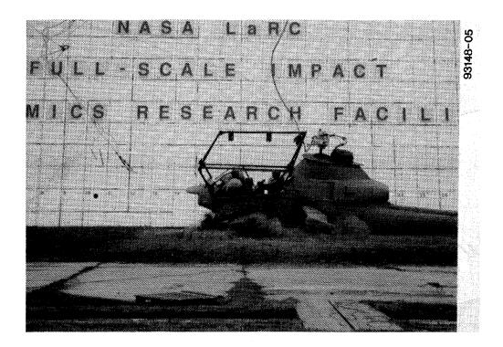
Figure 3: Aircraft Crash Test of IBAHRS and CABS
