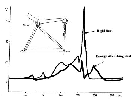
Fig. 2. Head Acceleration
