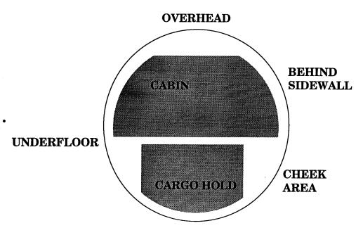
Figure 1 Cross Section of Fuselage Illustrating Hidden Areas
