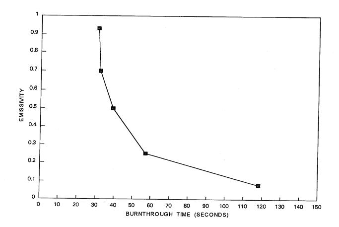
Figure 11 Surface Emissivity Against Burnthrough Time
