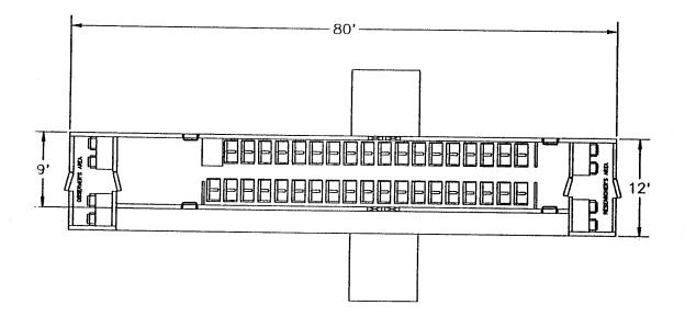
Figure 5 - Commuter Body Floor Plan
