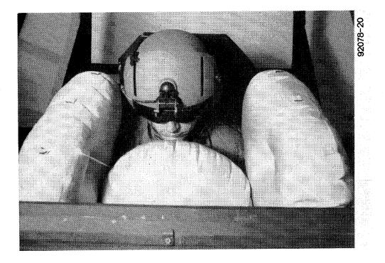
Figure 2: Cockpit Air Bag System
