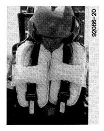
**Figure 1:** Inflatable Body and Head Restraint System
