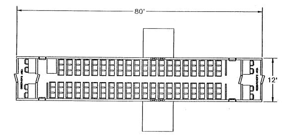
Figure 6 - Narrow Body Floor Plan
