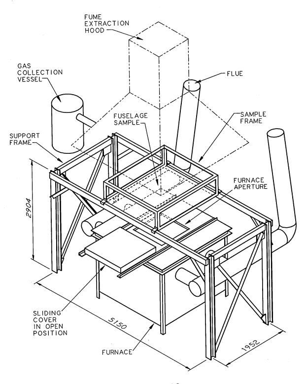
Figure 10 FUSELAGE BURNTHROUGH TEST FACILITY
