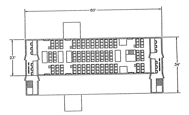
Figure 7 - Wide Body Main Deck Floor Plan
