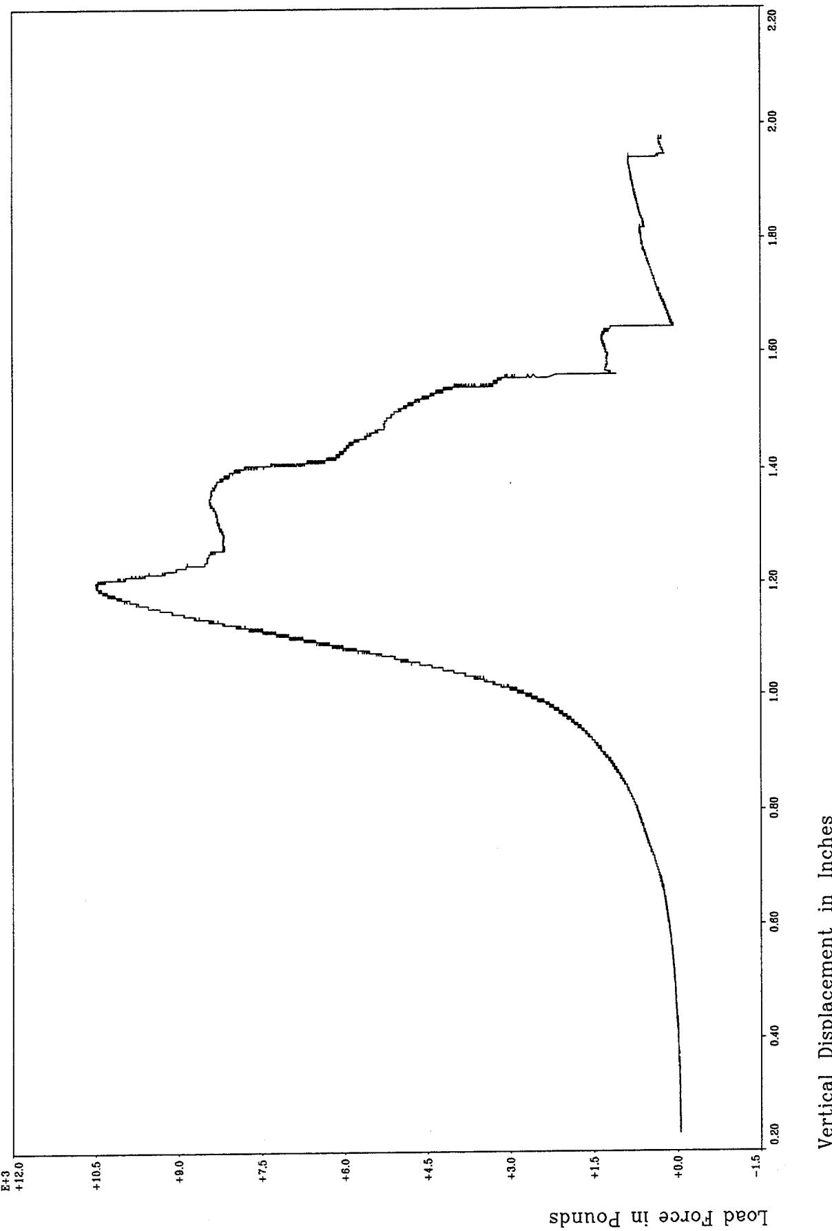
Test 5: 2 Inch Banding, 1 Seal (208 DG), 2 Crimps
