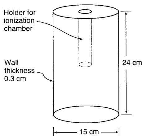
Fig. 3. Cylindrical phantom filled with TE liquid.
