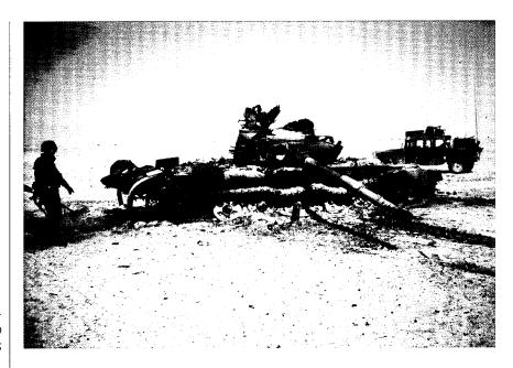
An Iraqi T-72 tank, penetrated and destroyed by two 120-mm. sabot rounds
