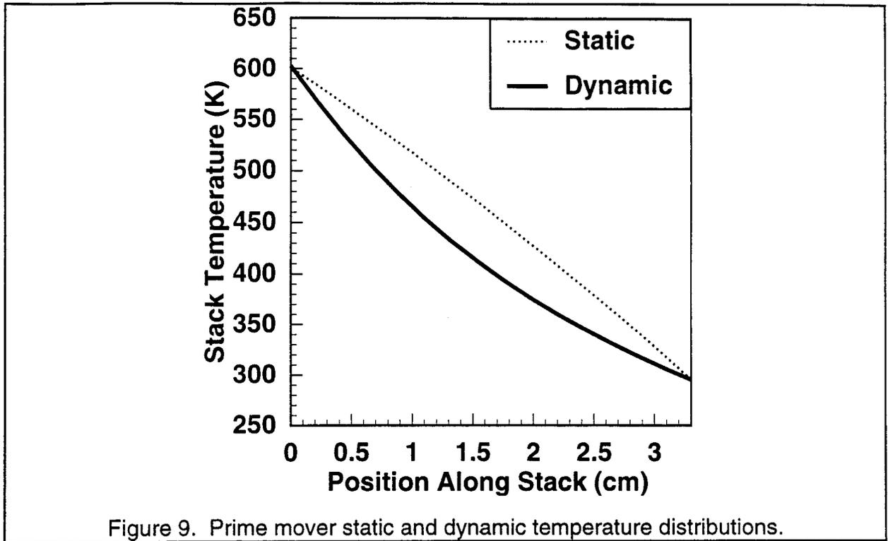
Figure 9 shows the static and dynamic temperature distributions in the prime mover stack. The static distribution occurs when no acoustic wave is present. The acoustic wave adds 2 extra path ways for heat transfer in the stack, in addition to thermal conductivity, as discussed in Ref. 2.
