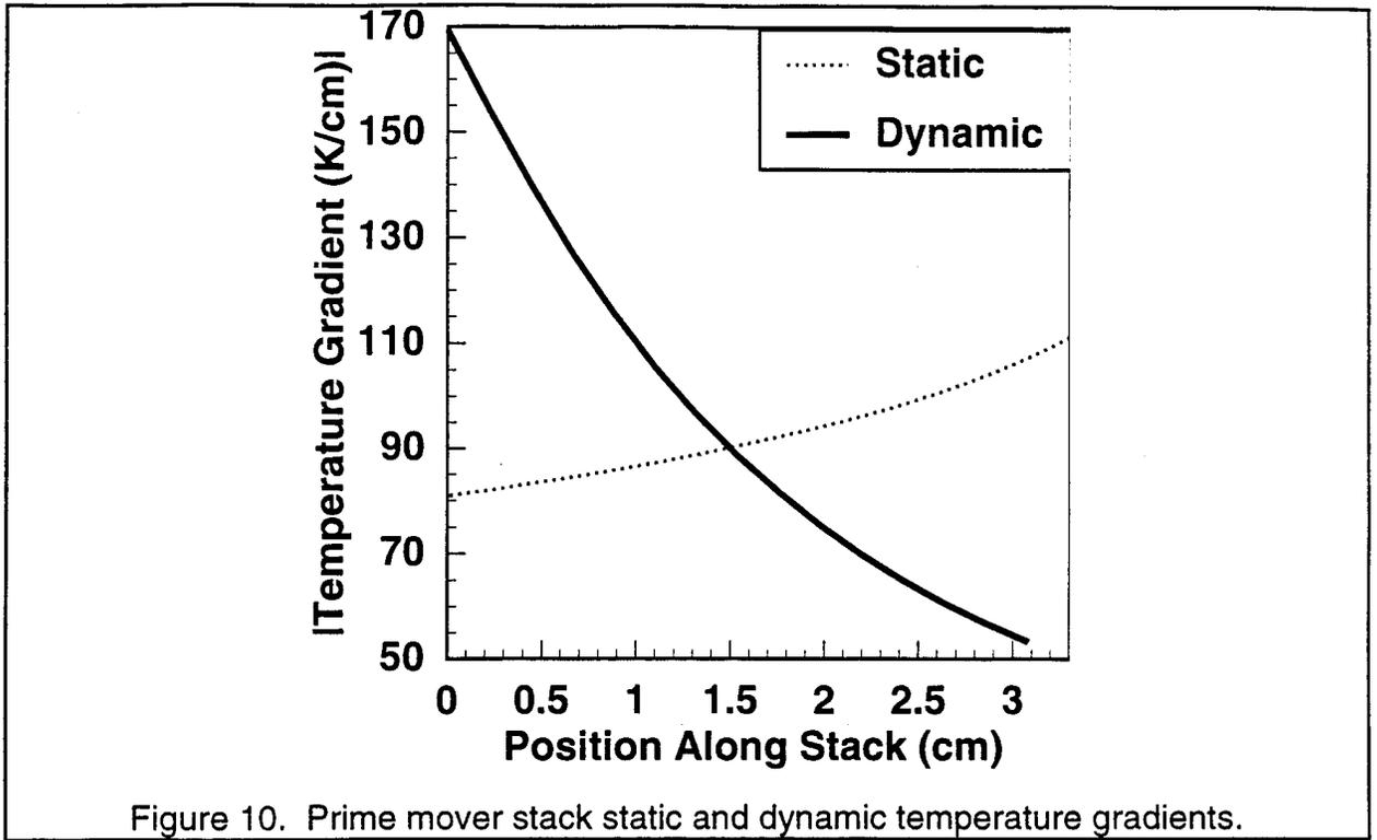
Thermoacoustic power generation in the stack is proportional to the gradient of temperature. Figure 10 shows that static and dynamic temperature gradients are quite different. The hottest end of the prime mover stack (see Fig. 8 for the temperature scale) has more than 3 times the temperature gradient of the cold end, indicating (all other things being equal), that thermoacoustic power generation in the stack is greatest at the hot end.
