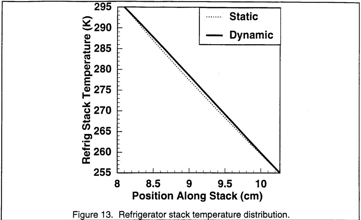
Figure 13 shows the refrigerator stack dynamical temperature distribution is similar to the static value.
