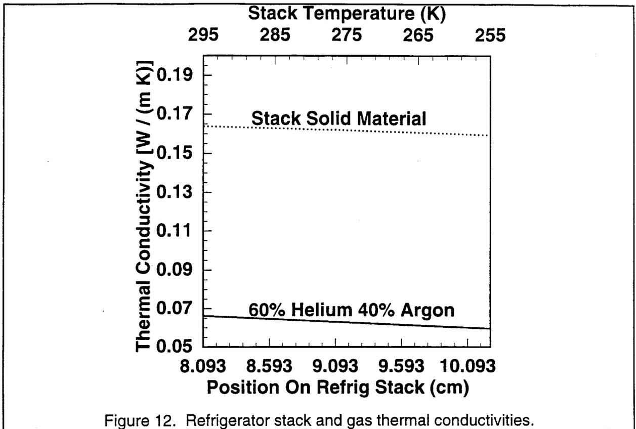
Figure 12. Refrigerator stack and gas thermal conductivities.
