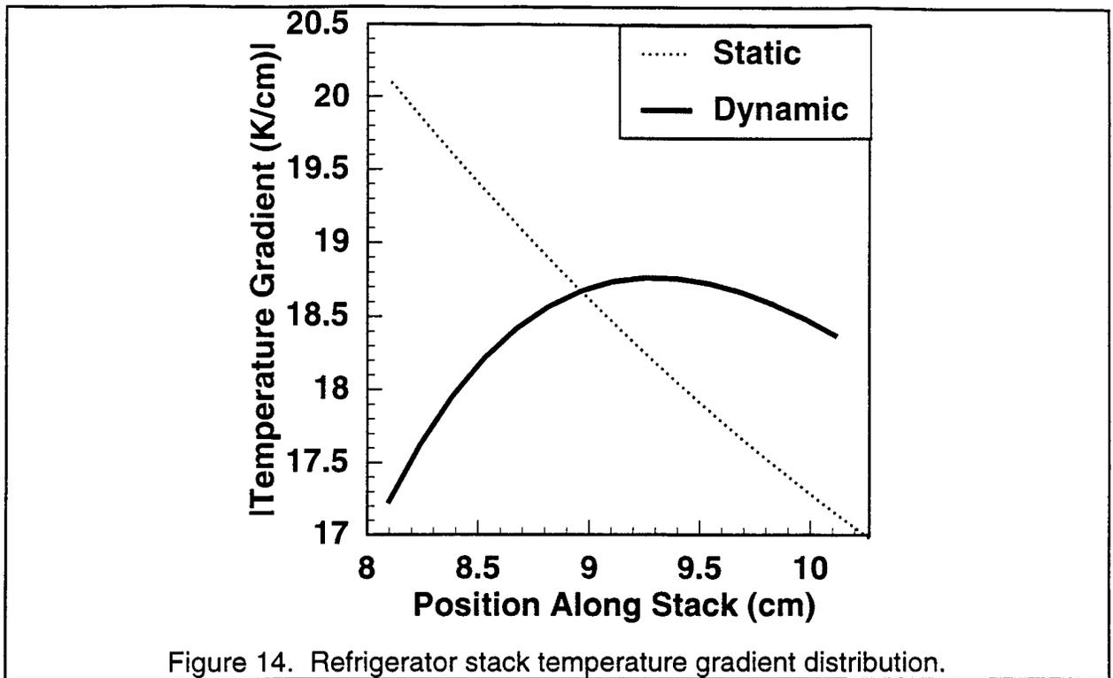
Figure 14 shows the radial stack temperature gradient. The short stack approximation indicates that acoustic refrigeration is greatest with no temperature gradient. The stack location and plate spacing somewhat diminish the dynamical gradient, though the effect is not pronounced.
