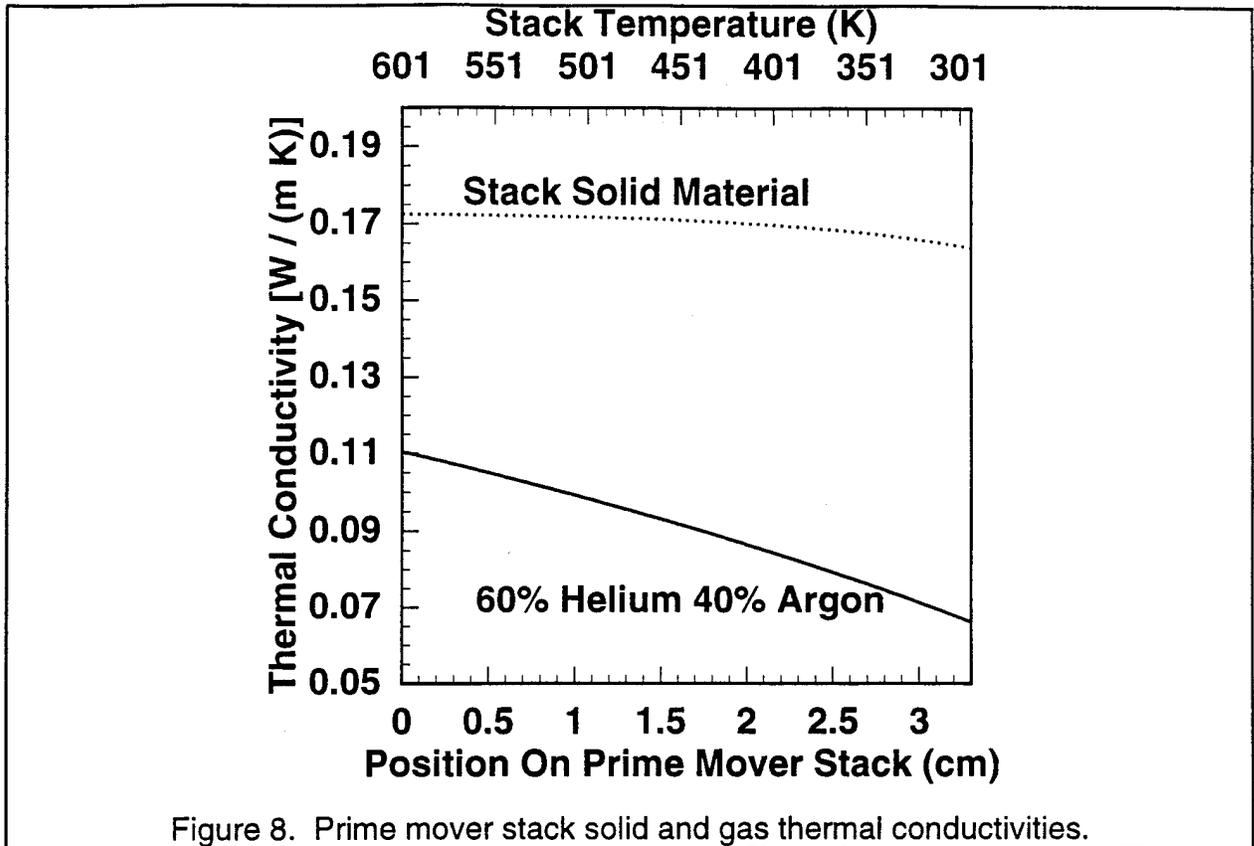
Figure 8. Prime mover stack solid and gas thermal conductivities.
