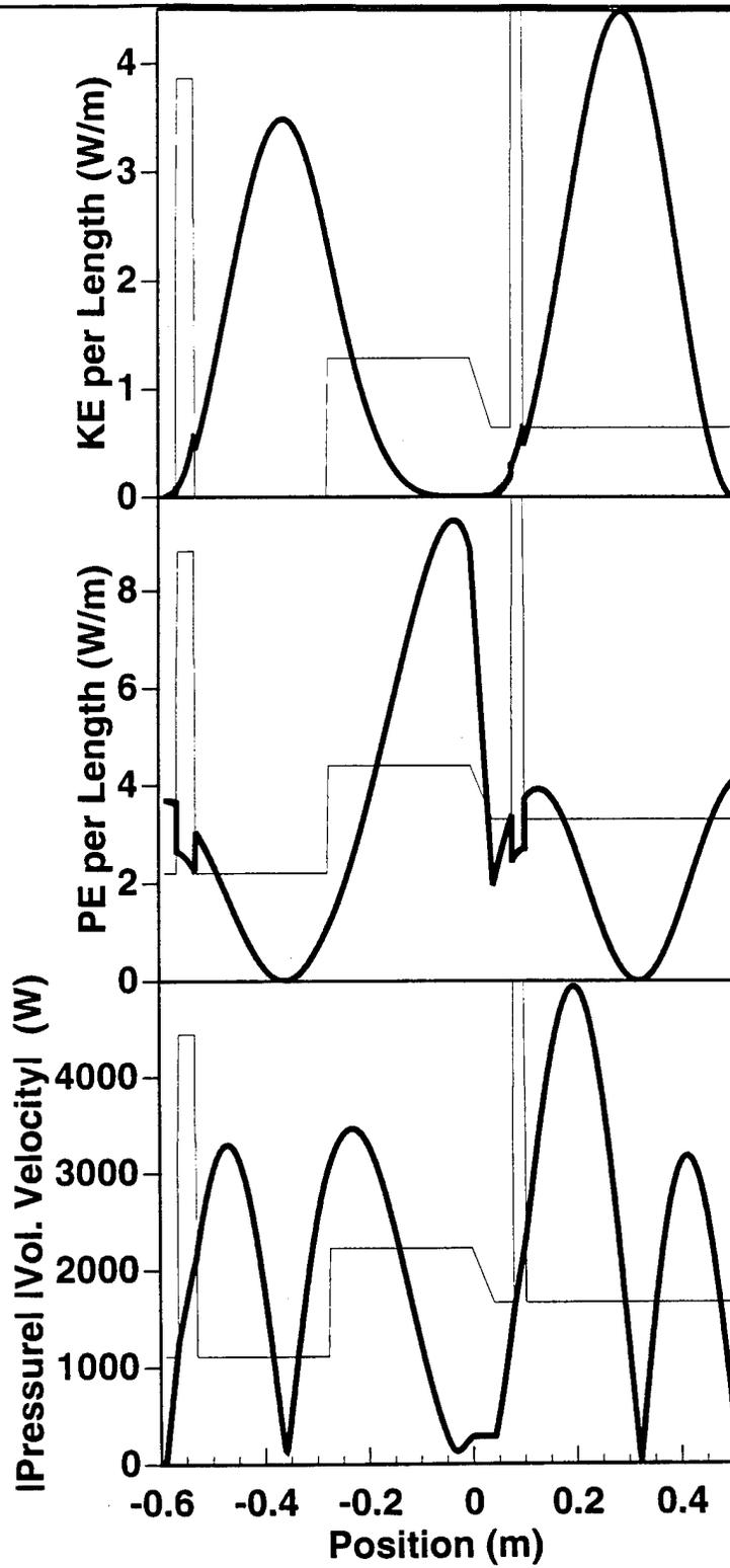
Figure 6. Kinetic, potential, and thermoacoustic power distributions.
