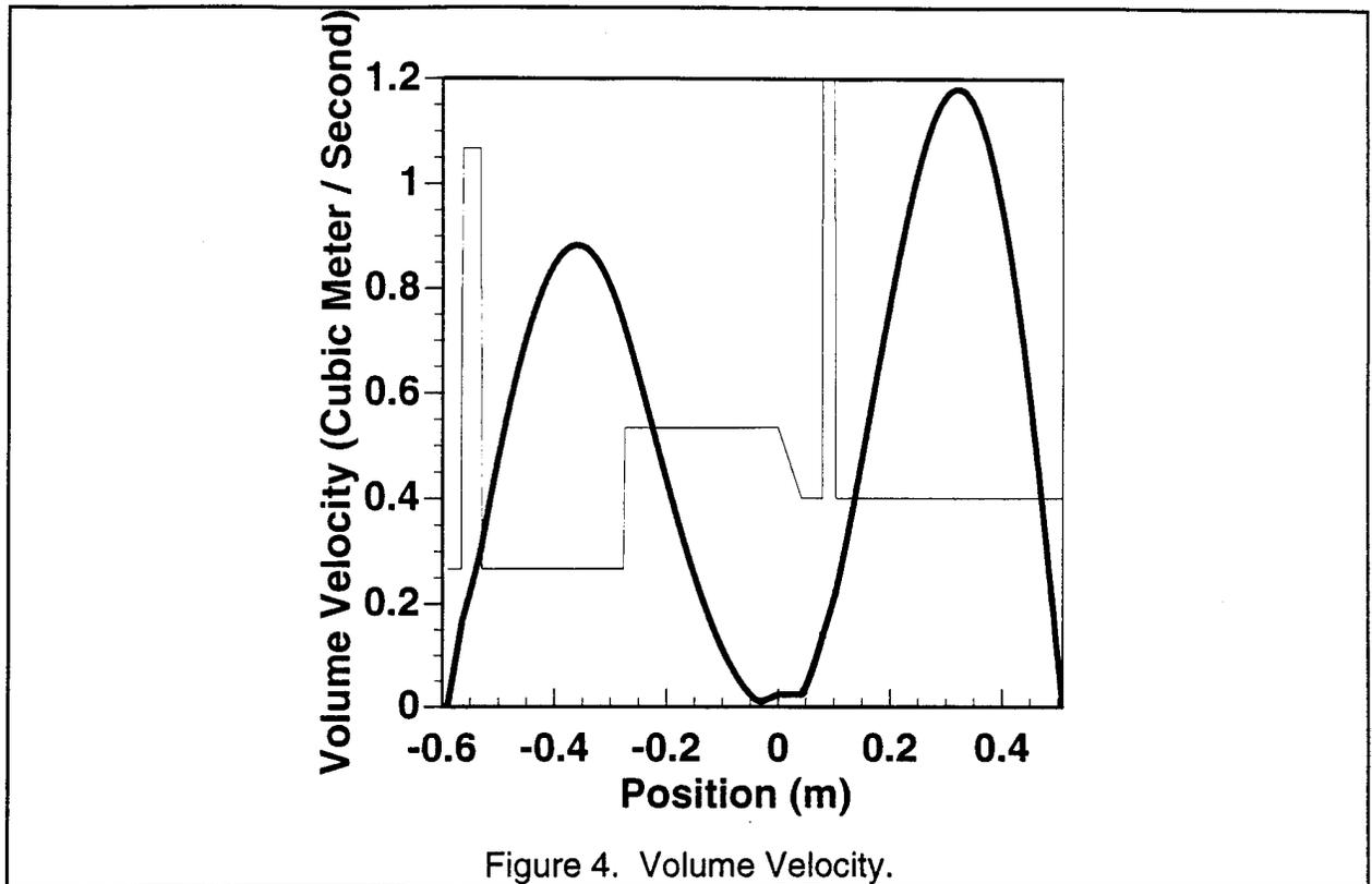
Figure 4 shows the volume velocity distribution. More than 1 cubic meter of gas oscillates per second through a radius of 0.3 m in the radial resonator. Stacks are at comparable volume velocities. The volume velocity is lowest at the transition from radial resonator to cone, purposely, to mode match the radial and plane wave resonators.
