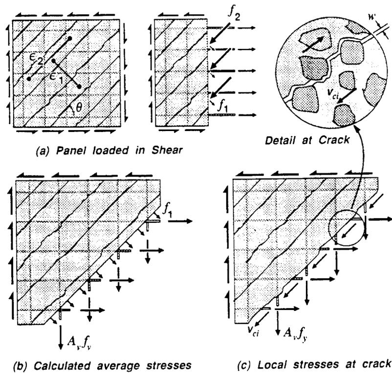
Figure 4. Reinforced concrete panels subjected to shear (Collins, 1996)
