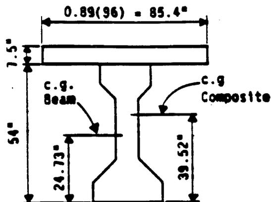
Figure 17. Transformed section of Girder Example IB (Feeser, 1994)
