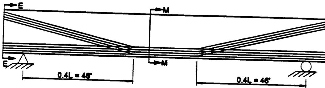
Figure 15. Prestressing Steel Harping Pattern Example IA (Feaser, 1994)
