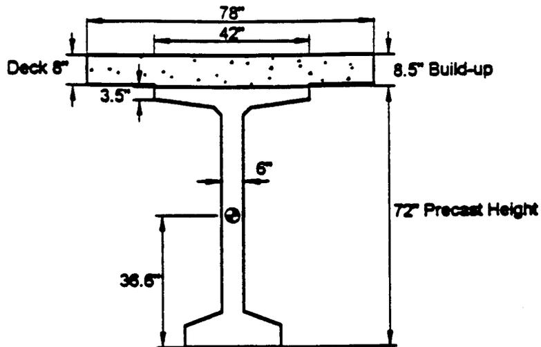
Figure 14. Girder Cross-Section Example IA (Feaser, 1994)
