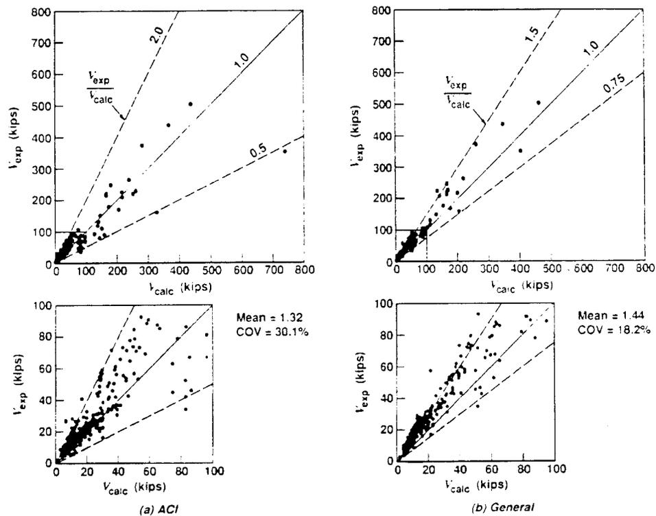
Figure 10. Experimental and predicted failure shears for 528 tests: ACI vs. General method (Collins, 1996).
