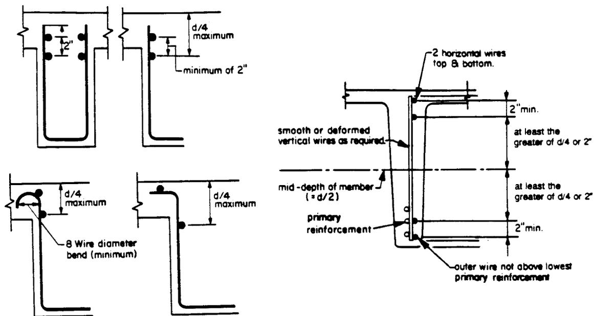
Figure 11. Anchorage of WWF in Concrete Beams (ACI 318-95)
