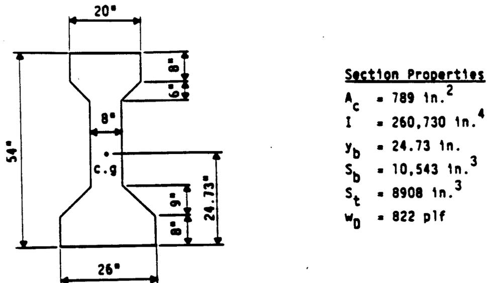
Figure 16. Cross Section of Girder Example IB (Feeser, 1994)
