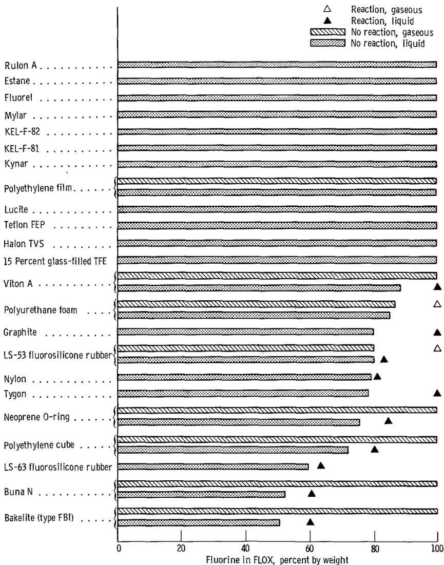
FIGURE 3-15.—Static compatibility test results for solid nonmetals in FLOX. Liquid FLOX temperature,  $-320^{\circ}\text{F}$ ; gaseous FLOX temperature,  $20^{\circ}$  to  $40^{\circ}\text{F}$ ; pressure, atmospheric (ref. 24). (These results should not be used as a guide in selecting materials to withstand dynamic conditions or pressures greater than atmospheric.)
