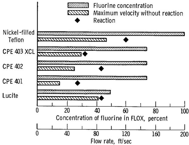
FIGURE 3-20.—Dynamic liquid FLOX compatibility tests (single data points, ref. 24). Pressure range, 100 to 400 pounds per square inch gage; temperature,  $-320^{\circ}\text{F}$ ; specimen configuration, 0.25-inch orifices.
