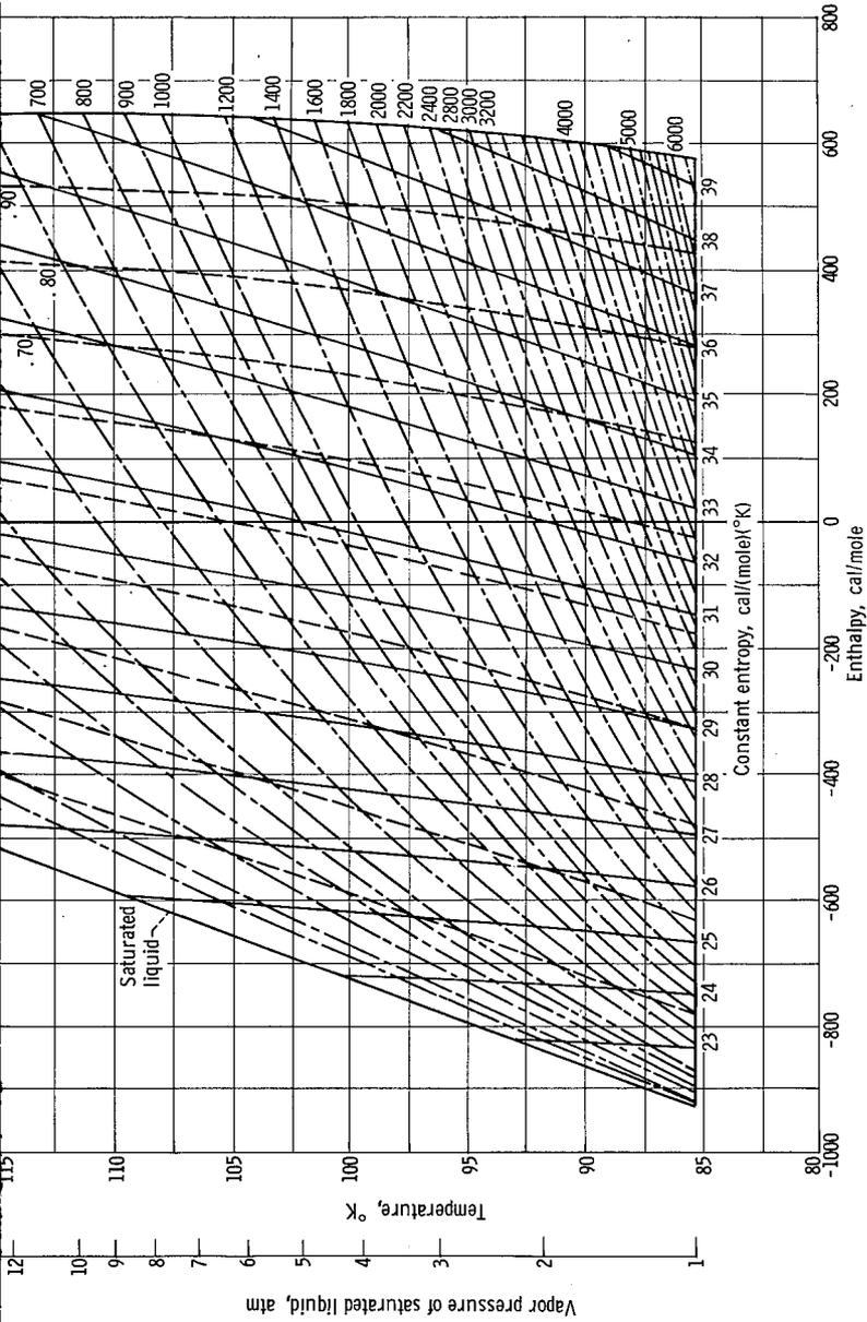
FIGURE 2-5.—Temperature-enthalpy diagram for fluorine (ref. 13).
