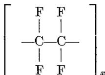
(2) FEP characteristics: Fluorinated ethylene propylene (FEP) tends to be more translucent (than TFE) at ambient conditions. It does not sublime like TFE, but becomes a very viscous fluid above a 500° to 530° F range. In addition, the material adheres to itself above this melting point range. The structure of the material is
