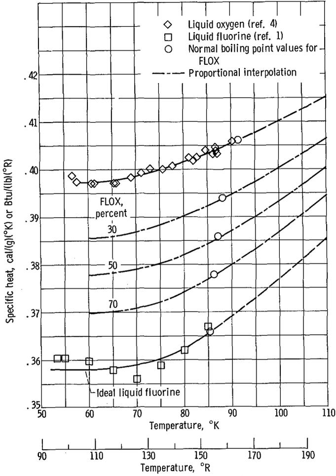
FIGURE 2-18.—Specific heat of liquid-fluorine-liquid-oxygen mixtures.
