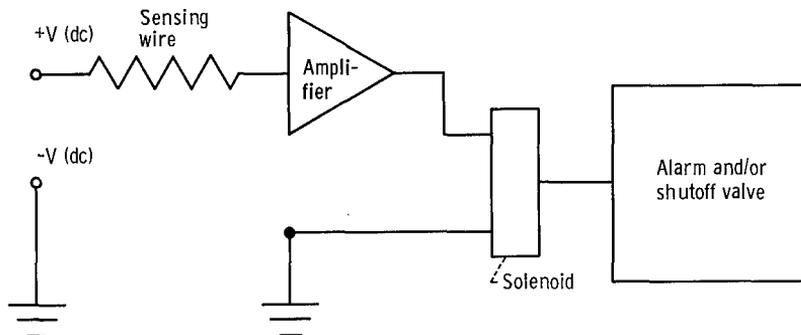
FIGURE 5-6.—Schematic drawing of burglar-alarm system.
