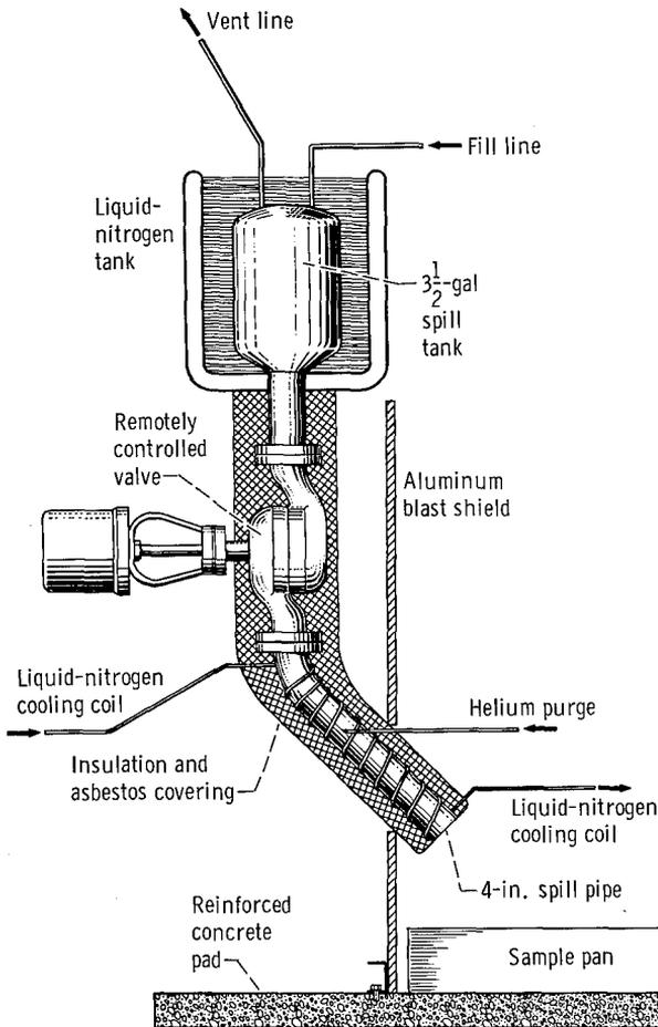
FIGURE 3-25.—Apparatus used for FLOX spill tests (ref. 25).
