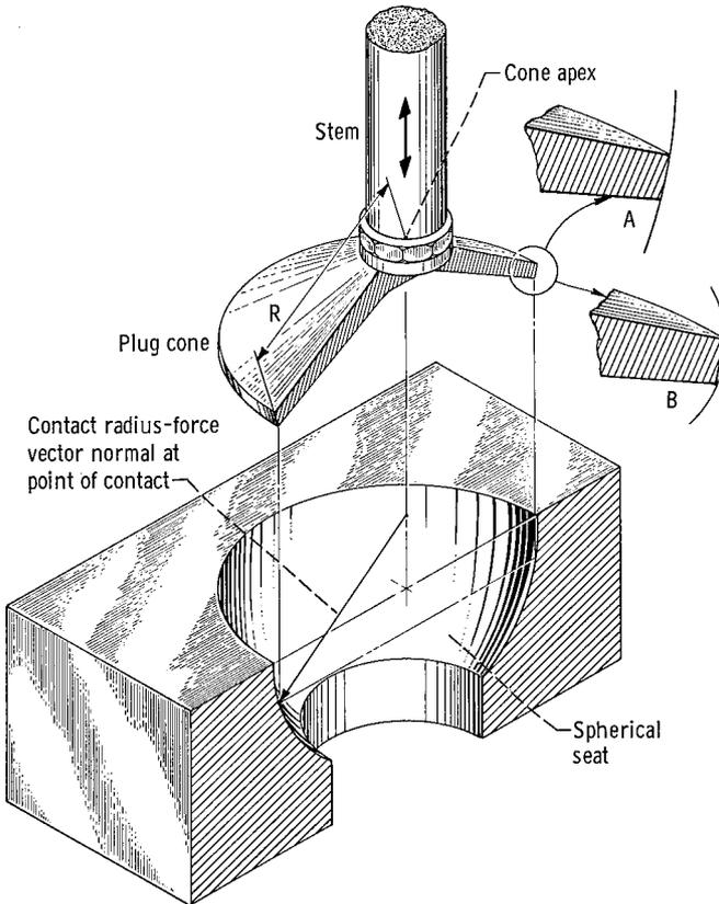
FIGURE 4-9.—Schematic drawing of conical valve design and operation.
