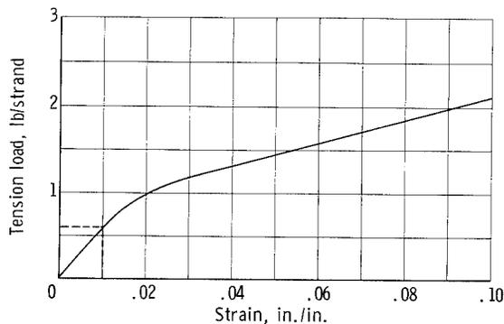
Figure 6. - Load-strain curve for single-strand nylon constrictive wrap.
