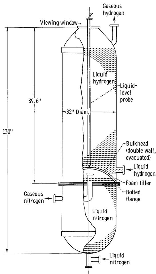
Figure 2. - Flight-weight propellant tank 2 used for insulation studies.
